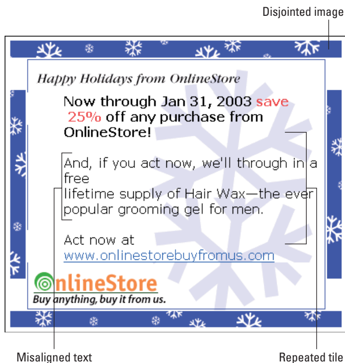
Figure 13-4: In Internet Explorer, this HTML page is stretched because the text is too large and forces the table cells to expand.
