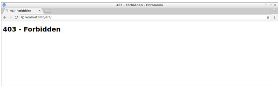
Figure 5-4. The HTTP 403 error status code displayed using the URL of a directory with no directory index and the directory listing disabled
