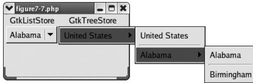
Figure 7-7. Two types of GtkComboBox widgets: GtkListStore gives a flat list (left), and GtkTreeStore presents a hierarchical structure (right)
