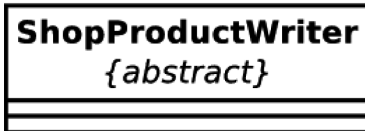
Figure 6-3. An abstract class defined using a constraint
