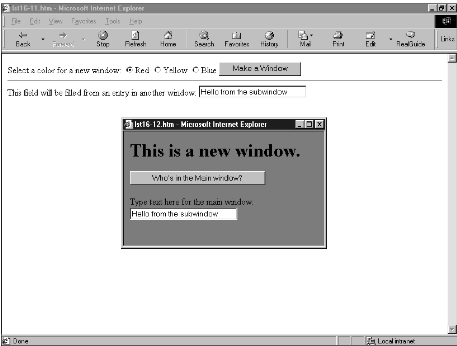
Figure 2-3: The main and subwindows, inextricably linked via the window.opener property
