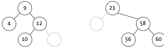
Figure 12-31: The third step: 12 is less than 20, so add to the left tree.
