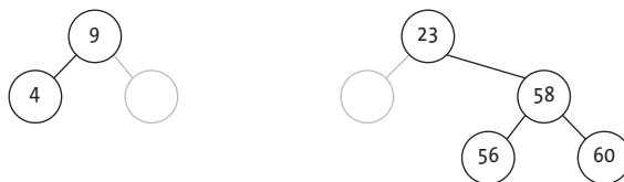
Figure 12-30: The second step: 9 is less than 20, so part of the tree goes to the left.
