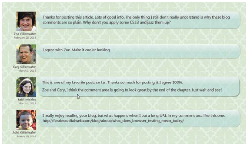
FIGURE 2.22 The larger shadow on hovered speech bubbles makes them appear to jump out at you a bit.
