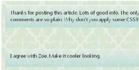
FIGURE 2.20 IE's Gradient filter can simulate simple CSS3 gradients (shown here in IE 8).
