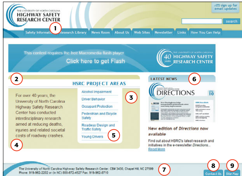
FIGURE 1.5 CSS3 abilities overrode the need for nine images, previously used in the numbered spots shown. The overall page looks about the same as it did in Figure 1.3.
