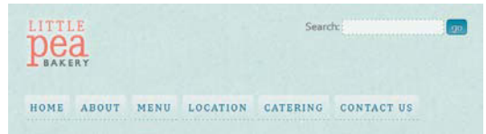
FIGURE 6.8 The nav bar can't fit beside the logo in narrow windows, so we switched it from the right side to the left using a media query.
