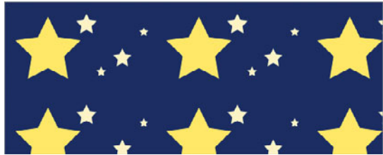
FIGURE 3.3 When the image is repeated across the background of the div , some of it gets cut off on the right and bottom.
