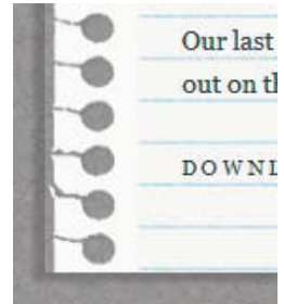
FIGURE 3.21 Drop shadows conform to the div's straight edge, not to any jagged lines within border or background images.
