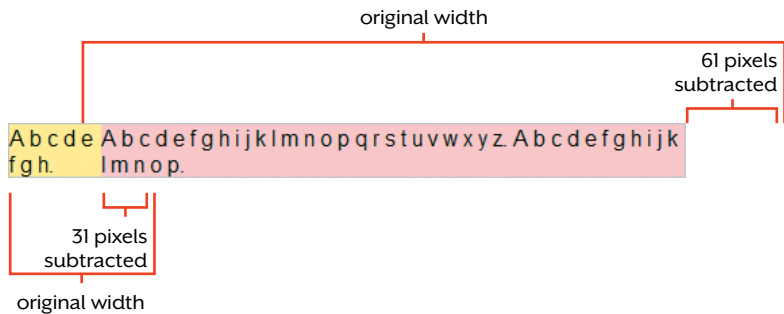
FIGURE 7.7 The pink div has 61 pixels subtracted from it, while the yellow one has only 31 pixels subtracted, since their box-flex values are in a two-to-one ratio.
