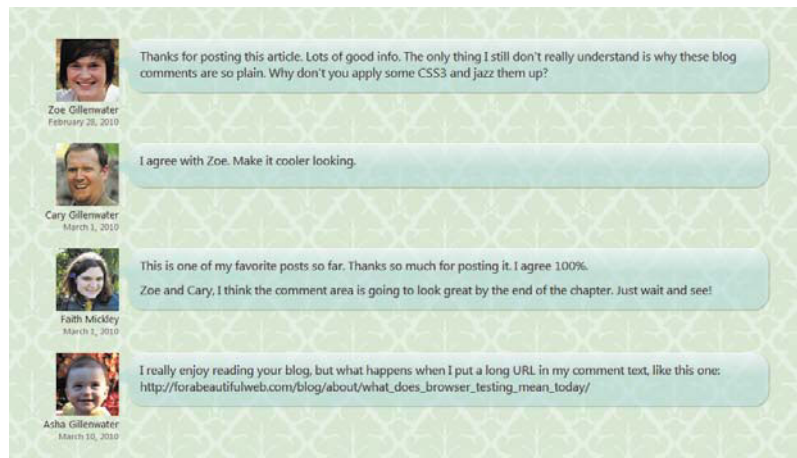
FIGURE 2.21 The box-shadow property adds a shadow beneath each speech bubble.
