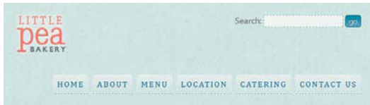
FIGURE 6.8 The nav bar can't fit beside the logo in narrow windows, so we switched it from the right side to the left using a media query.
