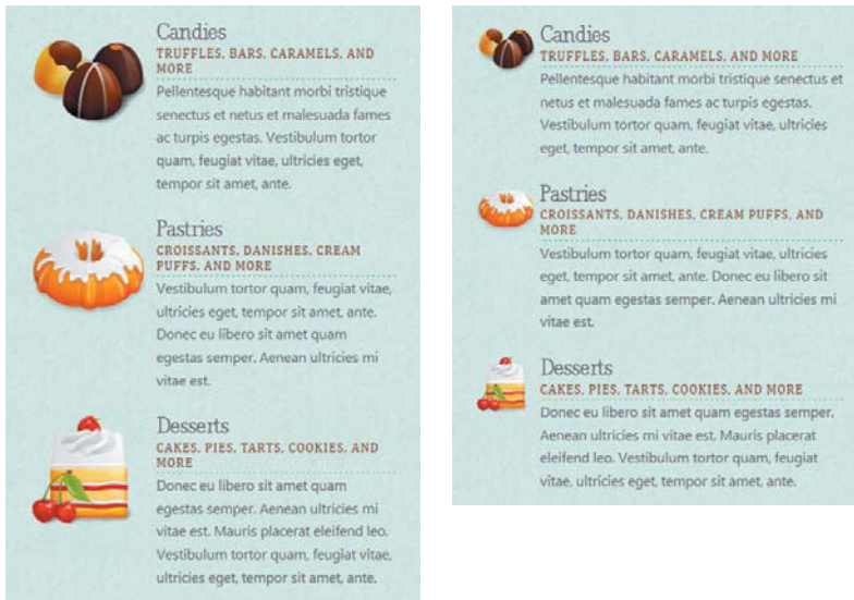
FIGURE 6.17 Reducing the size of the icons in the featured products area makes them look more balanced against the blocks of text in narrow widths.
