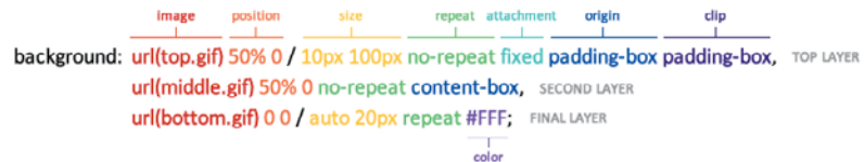
FIGURE 3.10 The background shorthand property can contain multiple layers; the top layer of this diagram includes all the possible pieces of the property (minus color, which can go only into the final layer).
