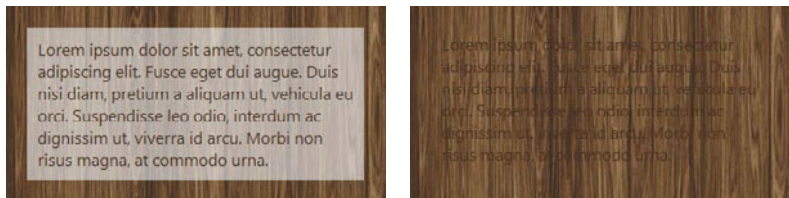
FIGURE 1.10 In Firefox (left), the box has a semitransparent background, but in IE 8 (right), no background appears, making the text unreadable.
