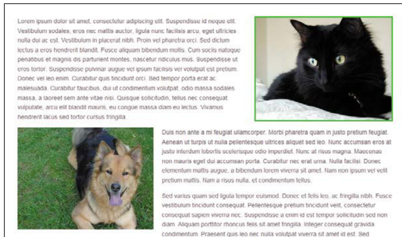
FIGURE 4.2 The image of the cat has an alt attribute on its img element, so it has a green outline. The image of the dog doesn't have an alt attribute.
