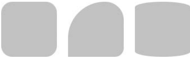
Figure 6-21. Many different shapes can be created by using the border-radius property.
