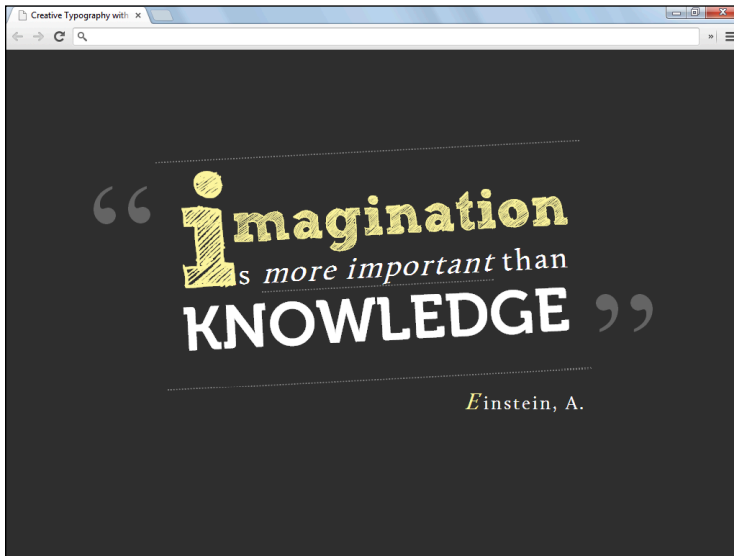
Figure 13-8 The quotation marks are added before and after the blockquote using the appropriate pseudo-elements.
