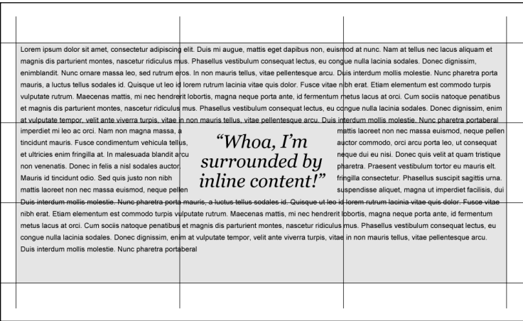
Figure 11-8 The wrap-flow: both; rule transforms the blockquote into an exclusion box and forces the text to wrap around it.
