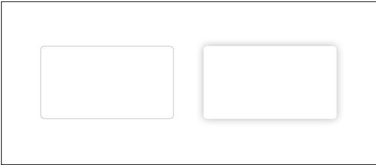
Figure 16-6 The modal window is given a light gray border (left), unless the box-shadow property/value pair is supported (right).
