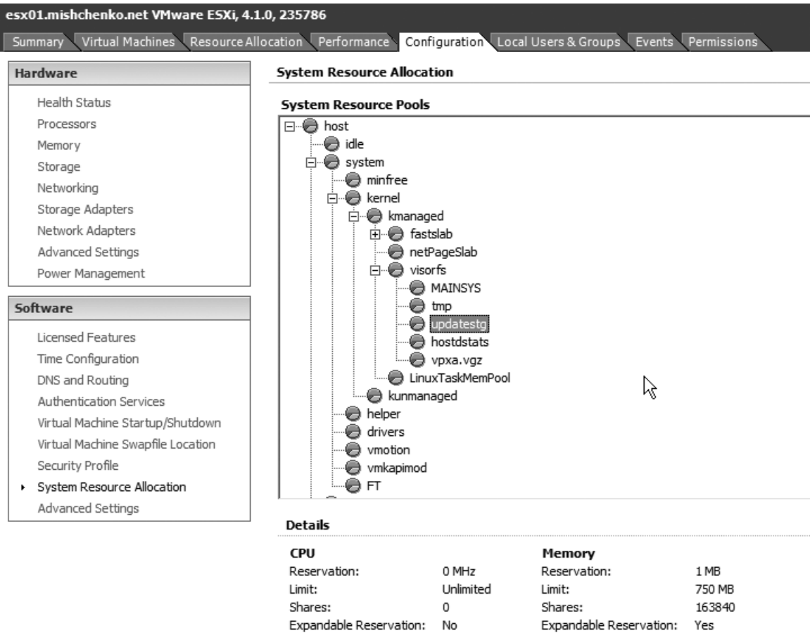
Figure 11.7 You can view resource allocation for the ESXi RAM disk filesystem with the System Resource Allocation screen.
