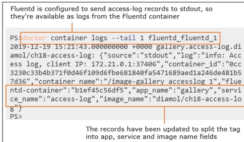
Figure 19.15 These logs are filtered so they're not stored in Elasticsearch but are echoed to stdout
