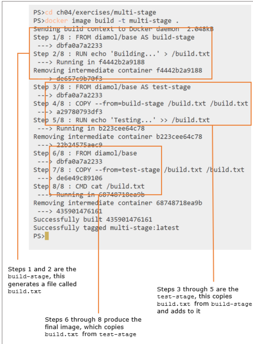
Figure 4.3 Building a multi-stage Dockerfile
