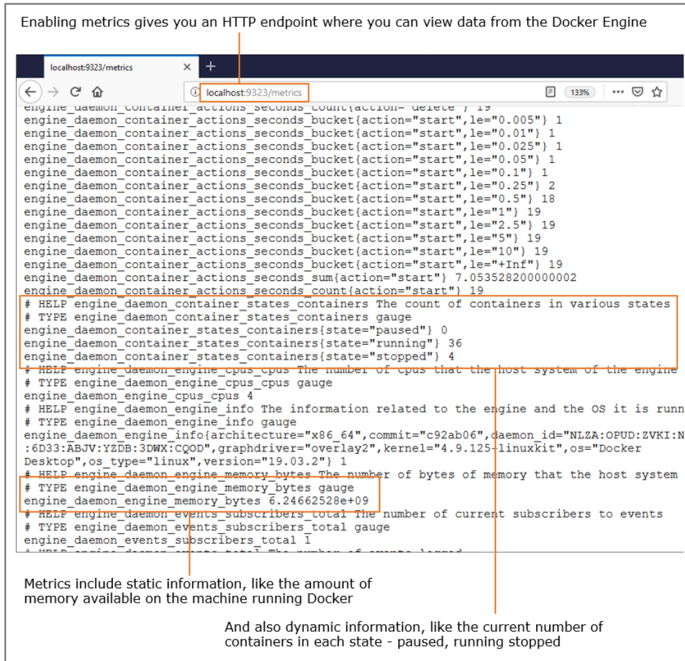
Figure 9.3 Sample metrics captured by Docker and exposed through the HTTP API
