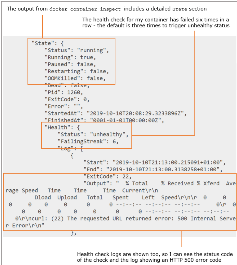
Figure 8.3 Containers with a health check show the health status of the app and the health check logs
