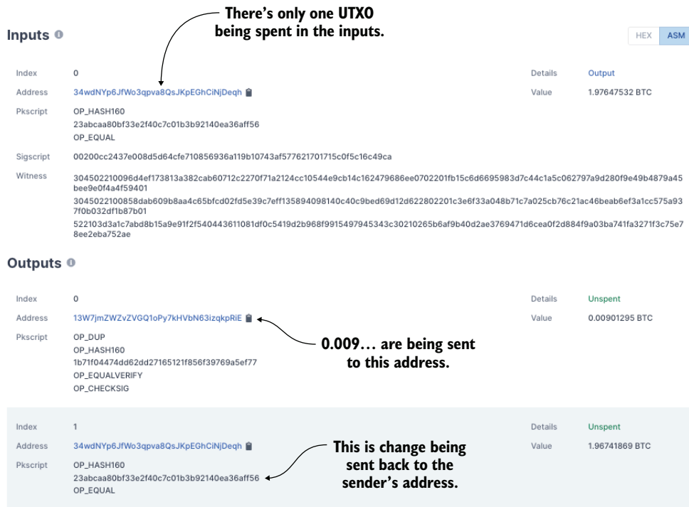
Figure 12.3 A random transaction I chose to analyze on https://blockchain.com ( http://mng.bz/n295 ). The transaction uses one input (of around 1.976 BTCs) and splits it in two outputs (of around 0.009 BTC and 1.967 BTCs). The difference between the total input amount and the total output amount is the transaction fee (not represented as an output). The other fields are the scripts written using Bitcoin's scripting language in order to either spend the UTXOs in the inputs or to make the UTXOs in the outputs spendable.
