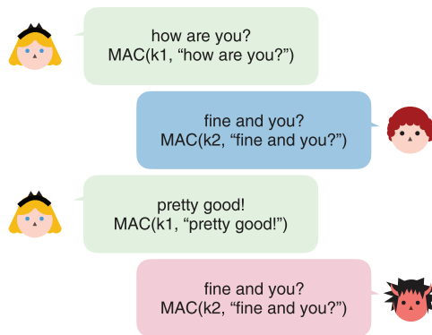
Figure 3.5 Two users sharing two keys, k_1 and k_2 , exchange messages along with authentication tags. These tags are computed from k_1 or k_2 , depending on the direction of the messages. A malicious observer replays one of the messages to the user.
