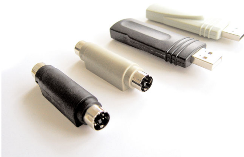
Figure 9-2 Assorted commercial USB and PS/2 key loggers (Courtesy: http://keyghostkeylogger.com/ )
