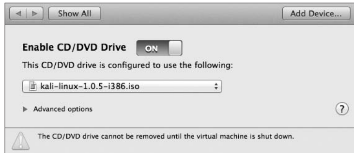
Figure 9-1: Setting our Windows 7 virtual machine to boot from the Kali ISO file
