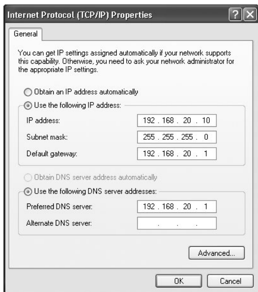
Figure 1-35: Setting a static IP address
