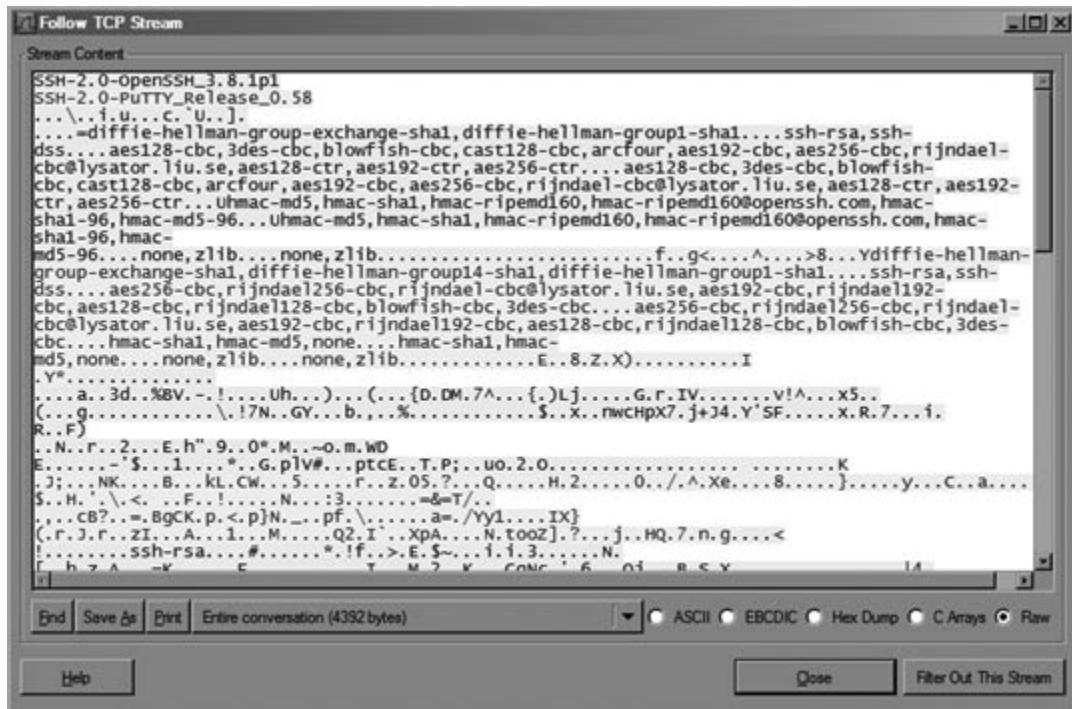
Figure 3.7 shows a packet capture from a SSH session. Note how the supported communication protocols are presented between the client and the server. Also note how the communication has been encrypted after the initial key exchange.
