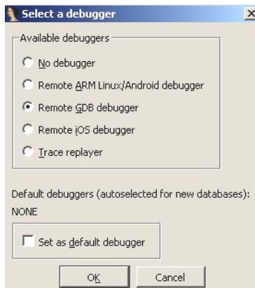
Figure 11.24 – Available debuggers for the 32-bit ARM sample in IDA
