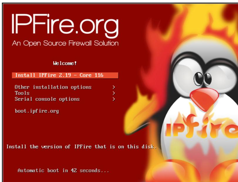
IPFire is completely free of charge, and it only takes a few minutes to set up. You install it on a machine with at least two network interface adapters and configure it to match your network configuration. It's a proxy type of firewall, which means that in addition to doing normal firewall-type packet inspection, it also includes caching, content filtering, and NAT capabilities. You can set up IPFire in a number of different configurations:
