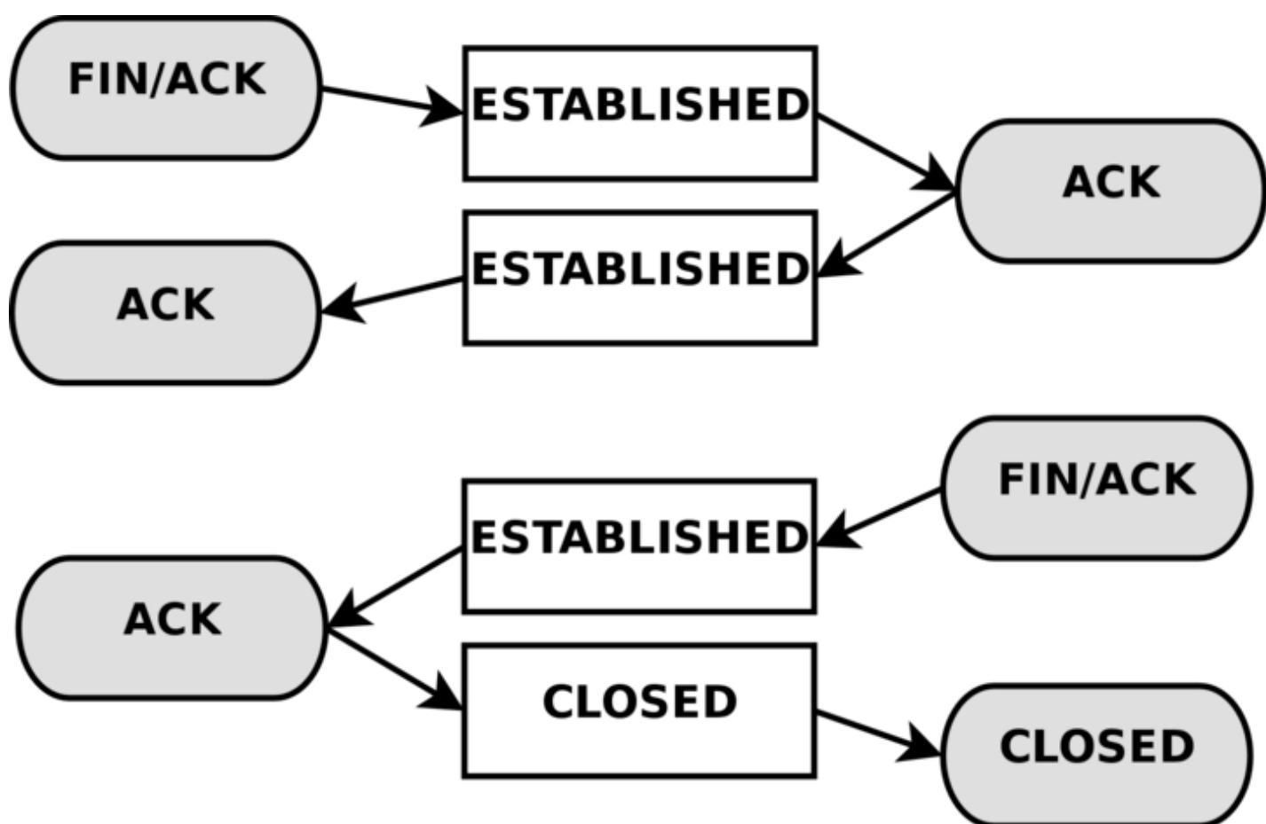
As you can see, the connection is never really closed until the last ACK is sent. Do note that this picture only describes how it is closed down under normal circumstances. A connection may also, for example, be closed by sending a RST(reset), if the connection were to be refused. In this case, the connection would be closed down immediately.
