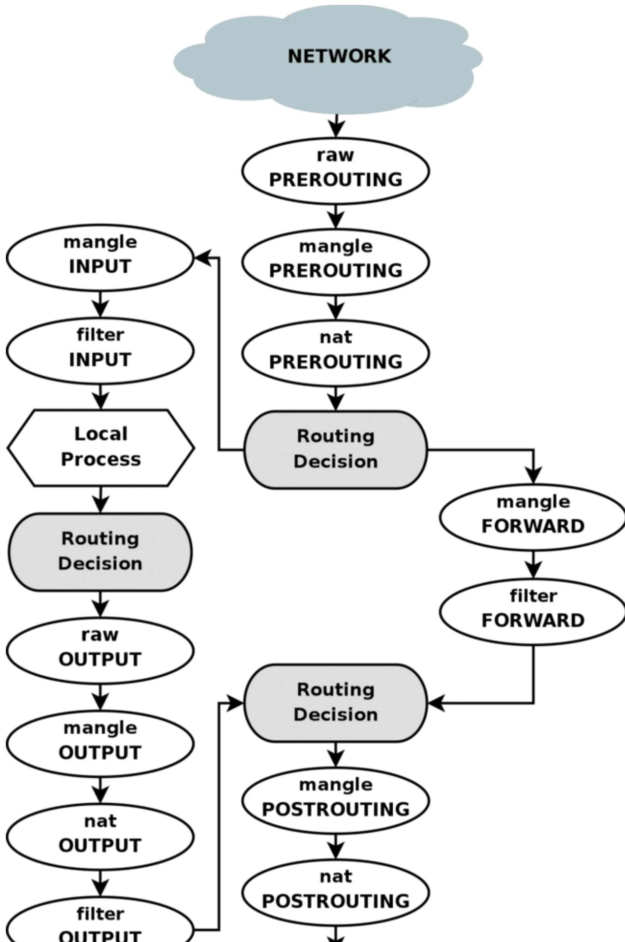
To clarify this image, consider this. If we get a packet into the first routing decision that is not destined for the local machine itself, it will be routed through the FORWARD chain. If the packet is, on the other hand, destined for an IP address that the local machine is listening to, we would send the packet through the INPUT chain and to the local machine.
