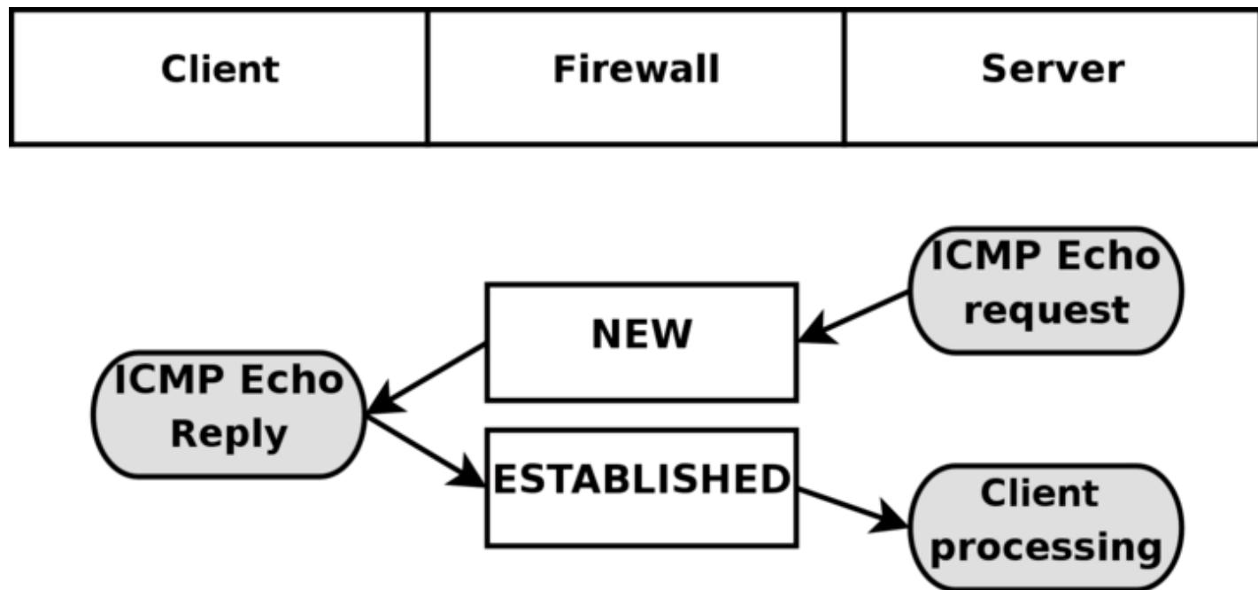
As you can see in the above picture, the host sends an echo request to the target, which is considered as NEW by the firewall. The target then responds with a echo reply which the firewall considers as state ESTABLISHED. When the first echo request has been seen, the following state entry goes into the `ip_conntrack`.
