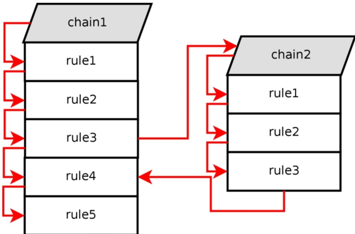
If one of the rules that matches points to another userspecified chain in the jump specification, the pointer will jump over to this chain and then start traversing that chain from the top to bottom. For example, see how the rule execution jumps from rule number 3 to chain 2 in the above image. The packet matched the matches contained in rule 3, and the jump/target specification was set to send the packet on for further examination in chain 2.
