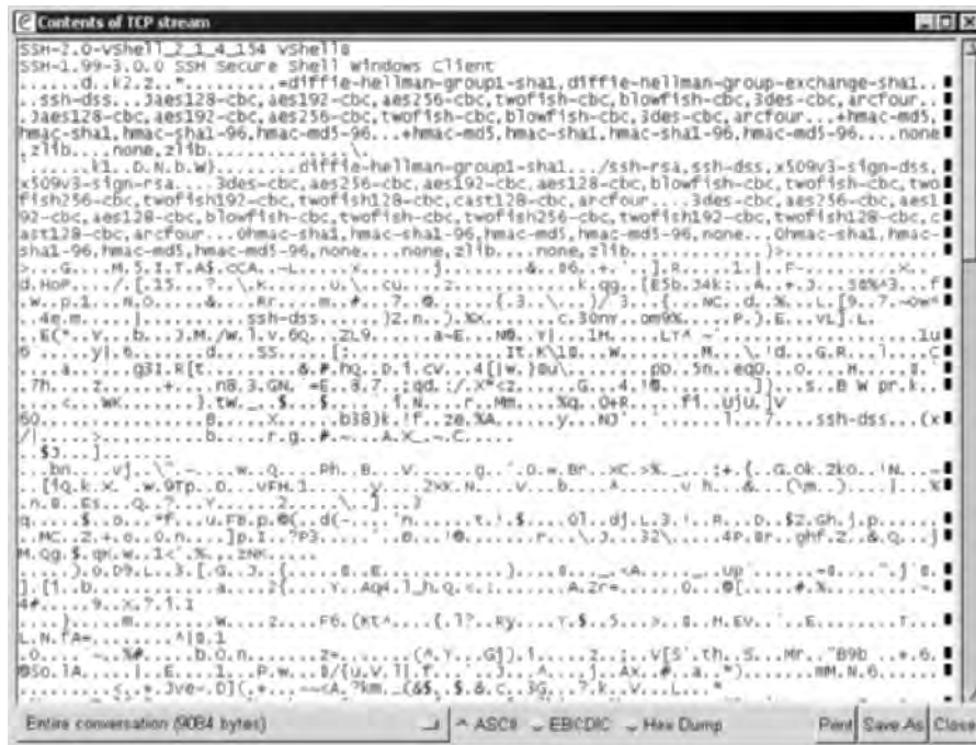
Figure 8.5 Sniffer program that captures an SSH connection.
