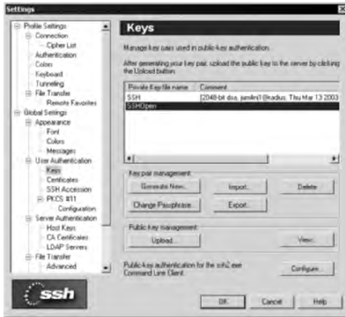
Figure 4.11 The SSH2 converted key in OpenSSH format in the SSH Communications' SSH GUI client.
