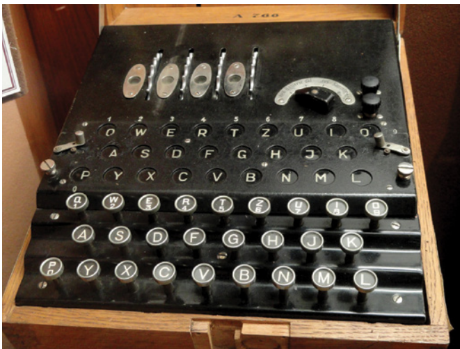
Figure 14.3: A German Enigma machine
