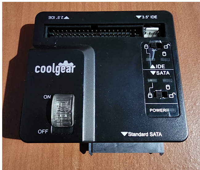
Figure 7.6 – USB to SATA and IDE write-blocker device
