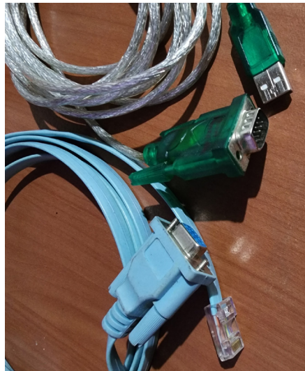
Figure 7.4 – Serial to JJ-45 (left) and Serial to USB (right) cables
