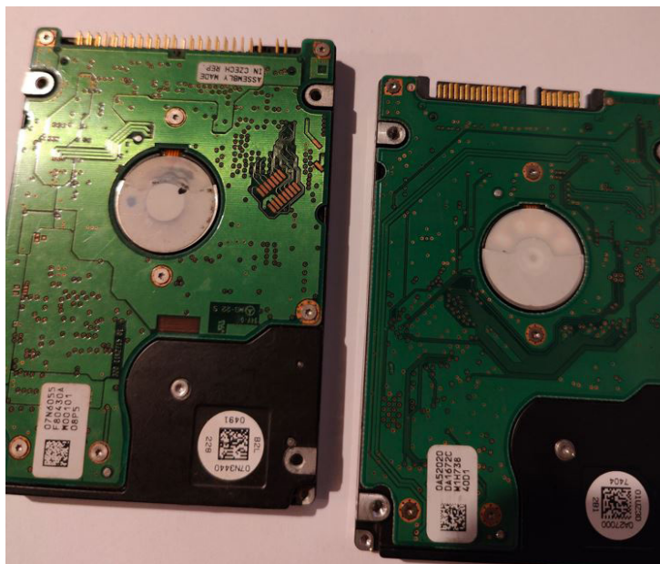
Figure 6.8 – 2.5-inch IDE (left) and SATA
