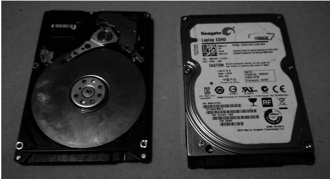
Figure 6.9 – Platters and actuator arm, which are housed in mechanical hard drives
