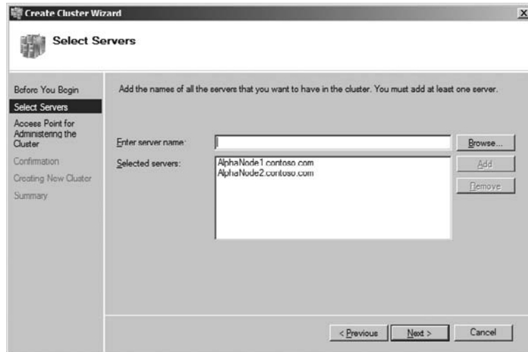
FIGURE 6.9 Enter all the nodes that are ready to join the cluster.
