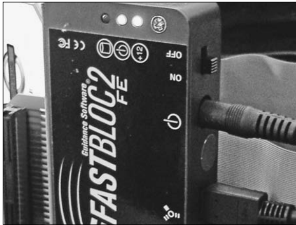
Figure 6-14: The write block device is powered up!
