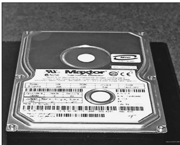
Figure 6-1: The classic magnetic- media hard drive.
