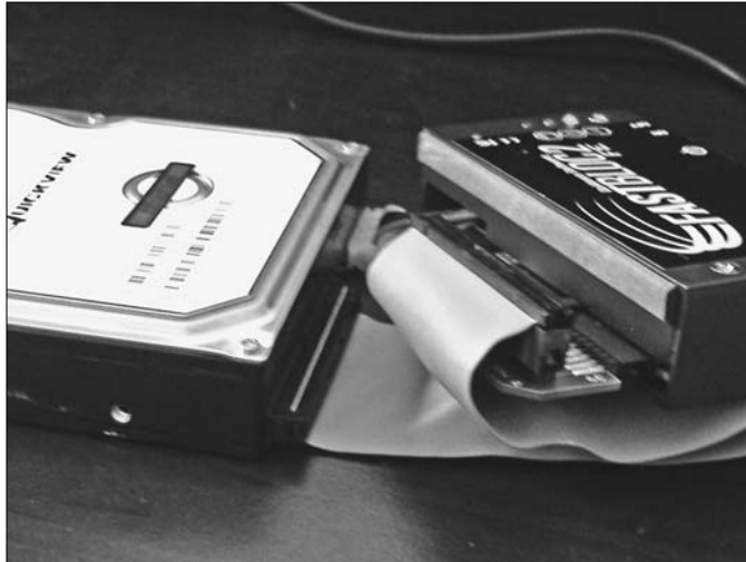
Figure 6-12: Connecting the EIDE adaptor to the write block device.
