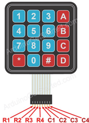
Figure 13.5 Pin configuration of the 4×4 keypad
