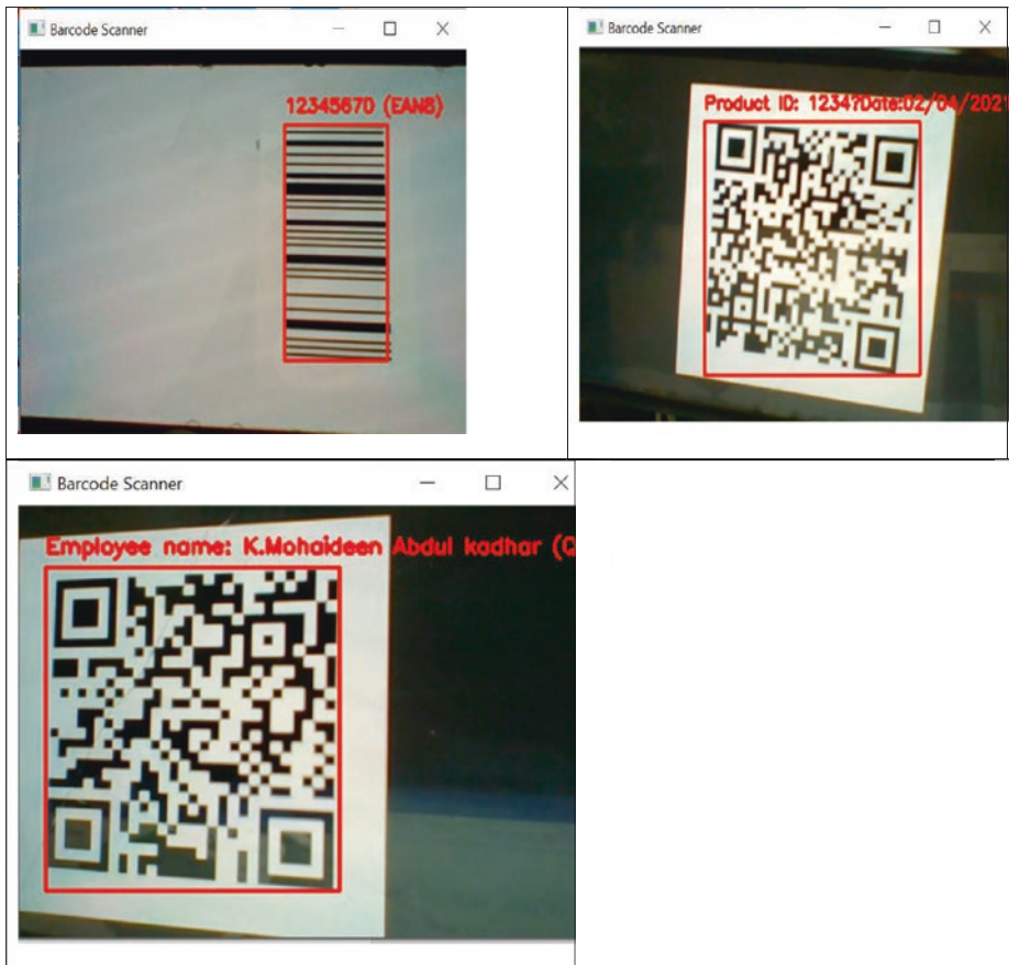
Figure 9-21. Output of barcode and QR code scanner
