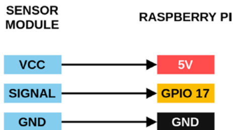
Figure 3-17. Temperature and humidity sensor with the Raspberry Pi GPIO pin
