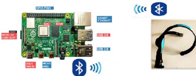
Figure 9-1. Raspberry Pi with MindWave Mobile connected via Bluetooth
