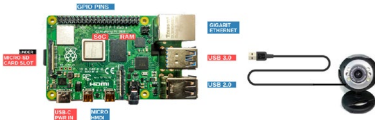
Figure 9-6. Raspberry Pi with webcam
