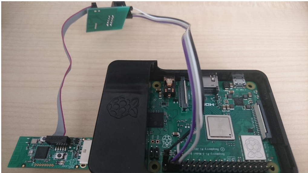
Figure 9.2 Connect the CC2531 and the downloader cable to the Raspberry Pi to flash new firmware to the USB sniffer.
