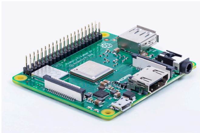
Figure 2.2 The Raspberry Pi 3A+ is fine as a home automation gateway if you don't need Ethernet connectivity and one USB 2.0 port is enough.
