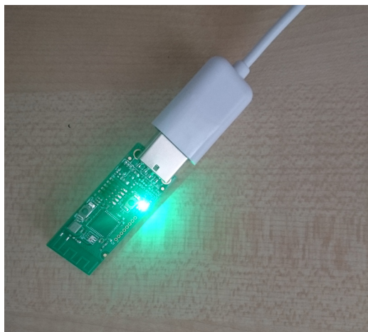
Figure 9.4 Connect the CC2531 with an USB extension cable to reduce interference from the Raspberry Pi's on-board Wi-Fi and Bluetooth.
