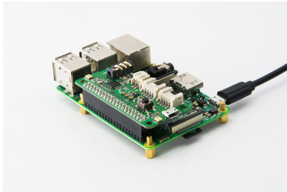
Figure 12.1 A Raspberry Pi with the ReSpeaker 2 Mics pHAT and a speaker (not shown here) is all you need to add voice control to your home automation system.
