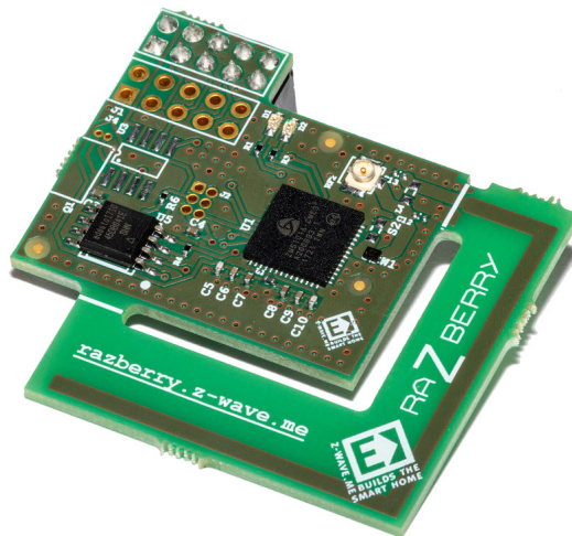
Figure 8.2 RaZberry is a tiny daughterboard with a Z-Wave controller chip that sits on top of the Raspberry Pi's GPIO header.
