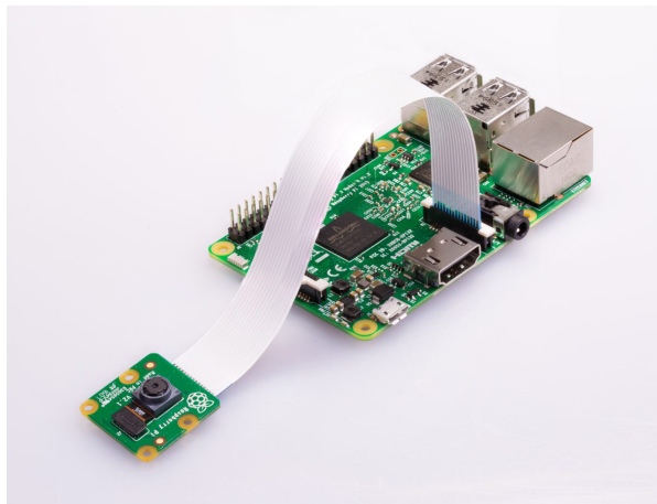
Figure 5.5 A Raspberry Pi with the Pi Camera Module makes an excellent IP camera.
