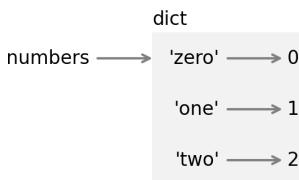
A dictionary is represented by a box with the word `dict` outside and the items inside. Each item is represented by a key and an arrow pointing to a value. The quotation marks indicate that the keys here are strings, not variable names.
