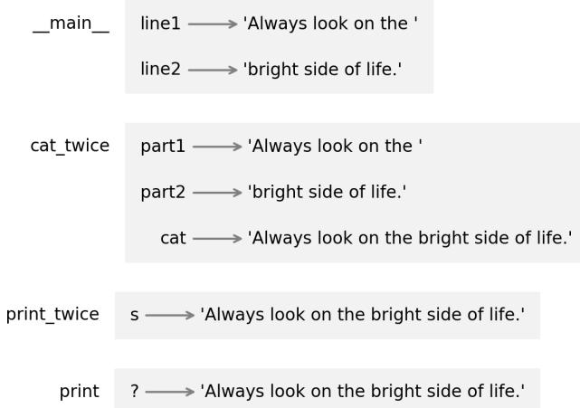
The frames are arranged in a stack that indicates which function called which, and so on. Reading from the bottom, `print` was called by `print_twice`, which was called by `cat_twice`, which was called by `__main__`—which is a special name for the topmost frame. When you create a variable outside of any function, it belongs to `__main__`.
