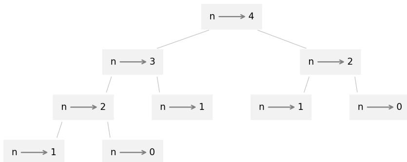
A call graph shows a set of function frames, with lines connecting each frame to the frames of the functions it calls. At the top of the graph, `fibonacci` with  $n=4$  calls `fibonacci` with  $n=3$  and  $n=2$ . In turn, `fibonacci` with  $n=3$  calls `fibonacci` with  $n=2$  and  $n=1$ . And so on.
