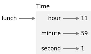
The variable `lunch` refers to a `Time` object, which contains three attributes. Each attribute refers to an integer. A state diagram like this—which shows an object and its attributes—is called an **object diagram**.
