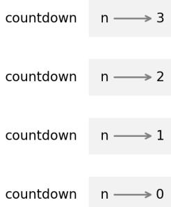
The four `countdown` frames have different values for the parameter `n`. The bottom of the stack, where `n=0`, is called the **base case**. It does not make a recursive call, so there are no more frames.
