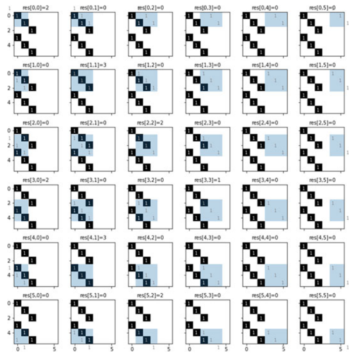
Fig. 4.74 The convolution process that produces the res array. As shown in the sequence, the light blue kern array is slid around, overlaid, multiplied, and summed upon the x array to generate the values of shown in the title. The output of the convolution is shown in Fig. 4.75
