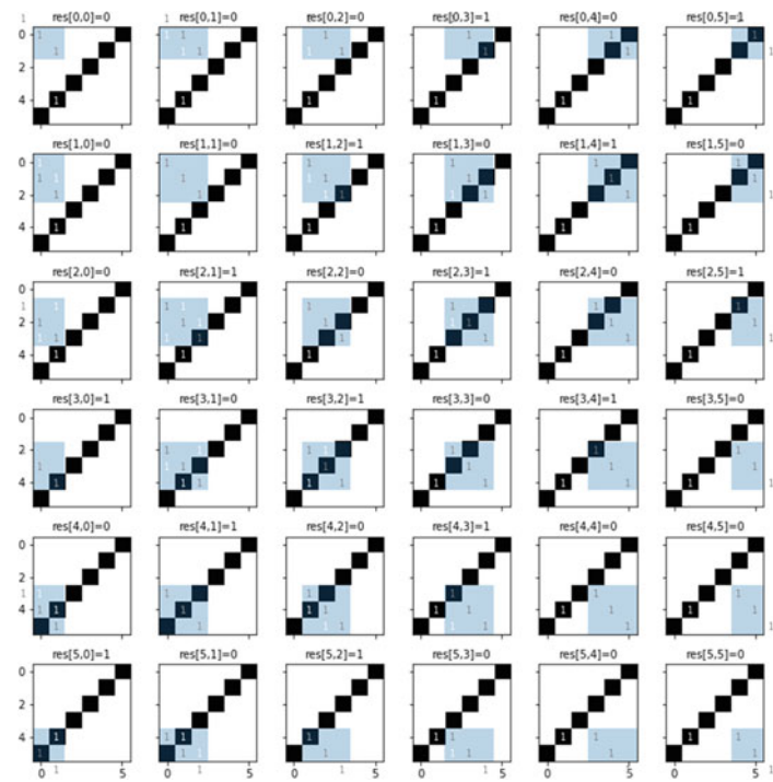
Fig. 4.76 The input array is a forward slash diagonal. This sequence shows the step-by-step convolution operation. The output of this convolution is shown in Fig. 4.77
