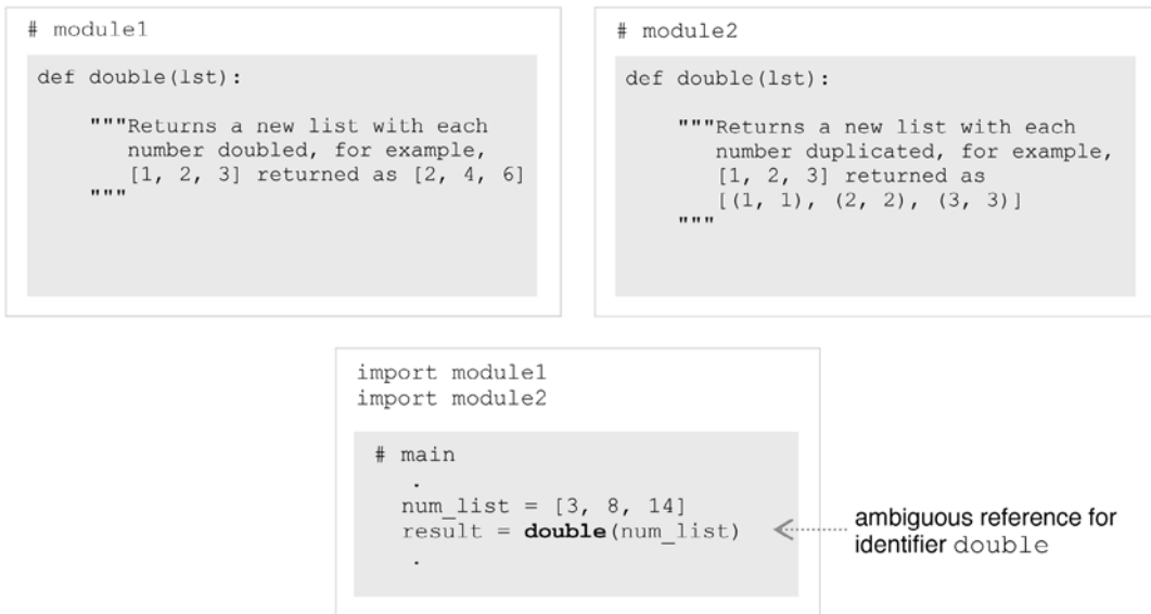
FIGURE 7-9 Example Name Clash of Imported Functions
