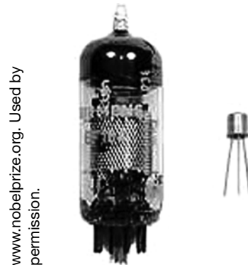
FIGURE 12-32 The Vacuum Tube vs. the Transistor
