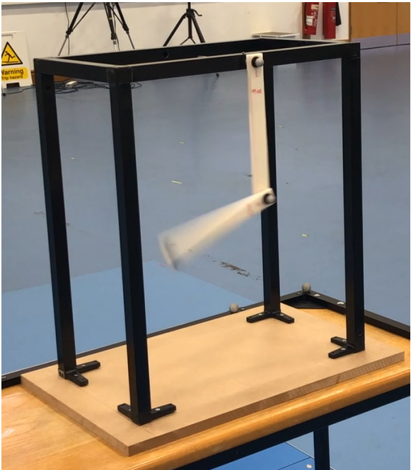
Fig. 4.10: A working double pendulum at the University of Hull (2019). Angle measurements were made using a high-speed motion-capture camera at the Sports Science Lab as part of an undergraduate research project. (Image credit: Mark Anguige.)
