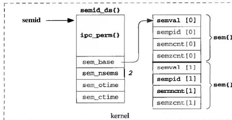
Figure 11.1 Kernel data structures for a semaphore set with two values in the set.
