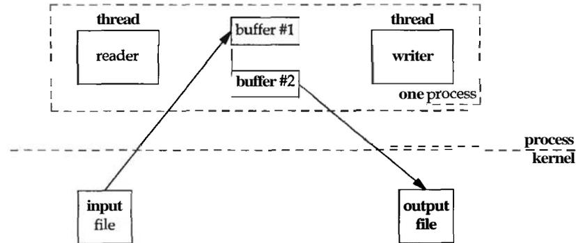
Figure 10.31 File copying divided into two threads using two buffers.
