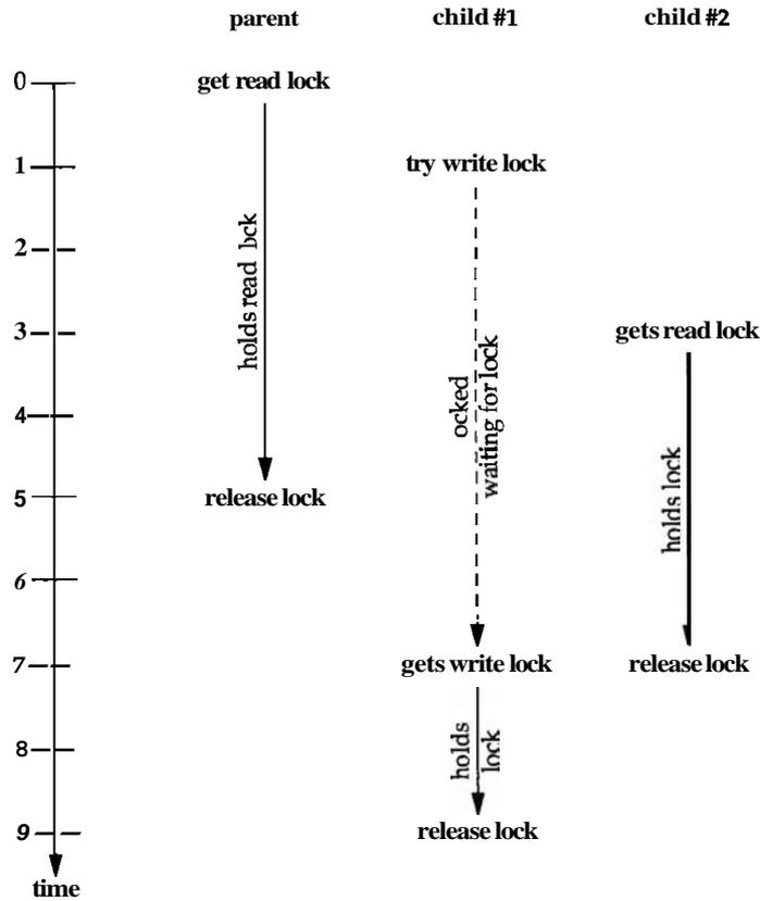
Figure 9.7 Determine whether another read lock is allowed while a write lock is pending.
