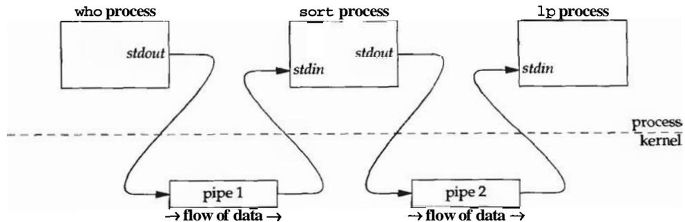
Figure 4.5 Pipes between three processes in a shell pipeline.
