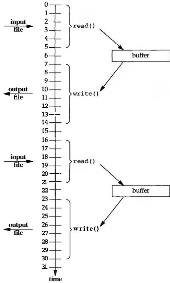
Figure 10.28 One process that reads data into a buffer and then writes the buffer out.
