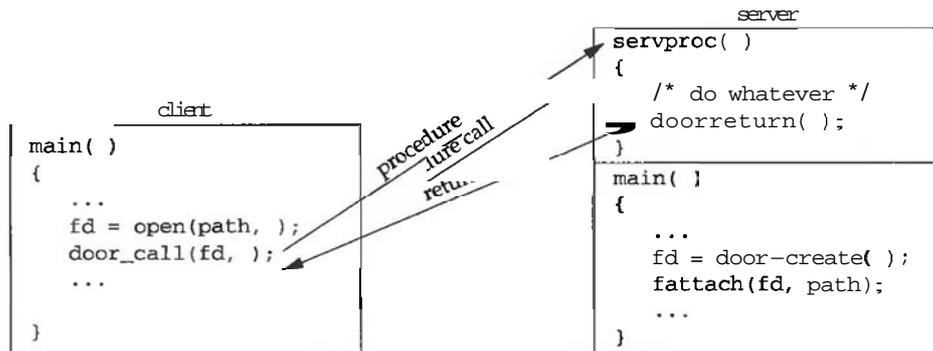
Figure 15.4 Apparent procedure call from one process to another.
