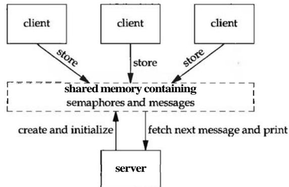
Figure 13.9 Multiple clients sending messages to a server through shared memory.
