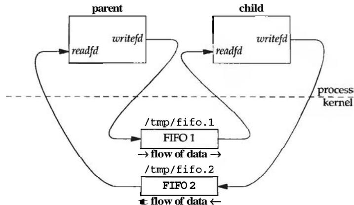
Figure 4.17 Client-server example using two FIFOs.
