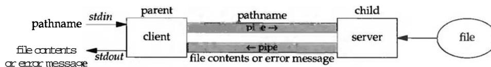
Figure 4.7 Implementation of Figure 4.1 using two pipes.
