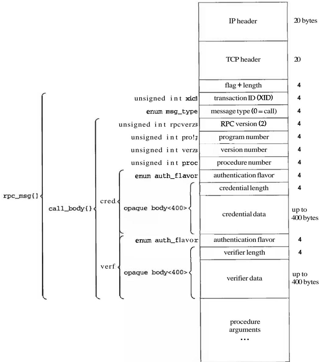
Figure 16.30 RPC request encapsulated in a TCP segment.
