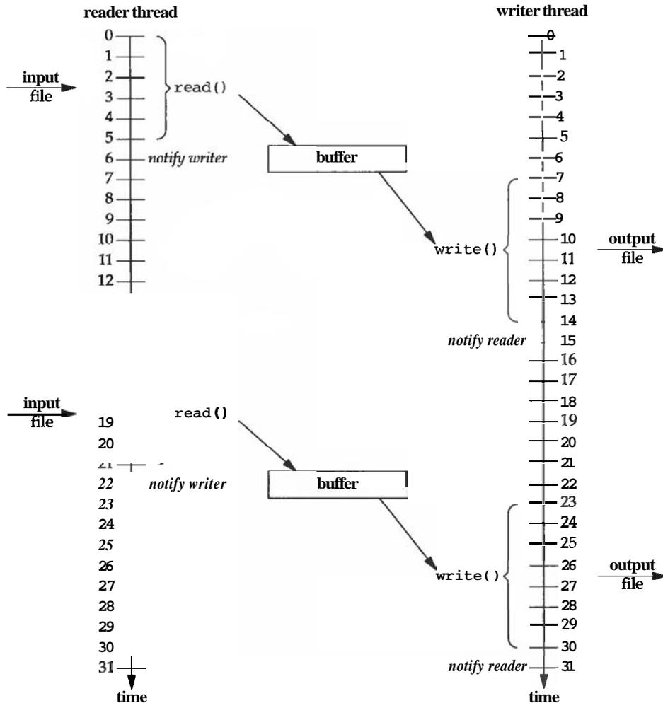
Figure 10.30 File copying divided into two threads.
