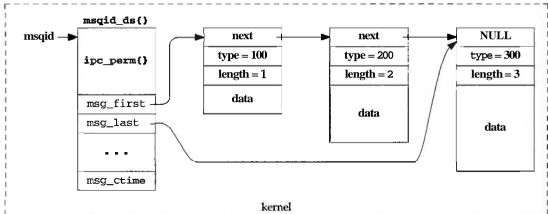
Figure 6.1 System V message queue structures in kernel.
