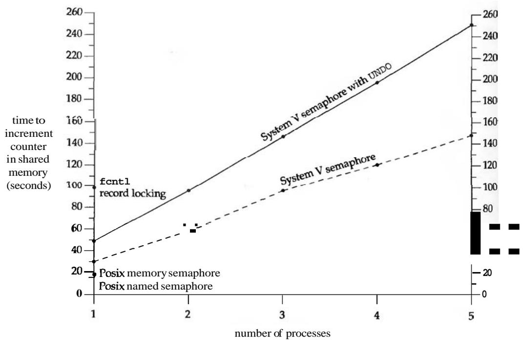
Figure A.13 Time required to increment a counter in shared memory (Digital Unix 4.0B).
