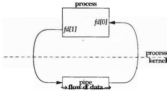
Figure 4.2 A pipe in a single process.
