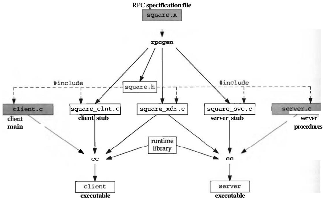
Figure 16.4 Summary of steps required to build an RPC client-server.
