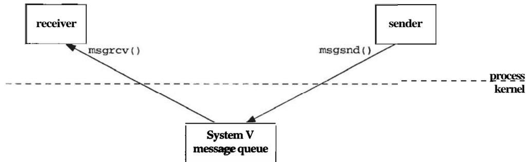
Figure D.7 Sending messages using a System V message queue.
