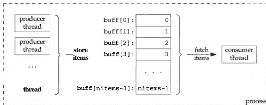
Figure 7.1 Producer-consumer example: multiple producer threads, one consumer thread.
