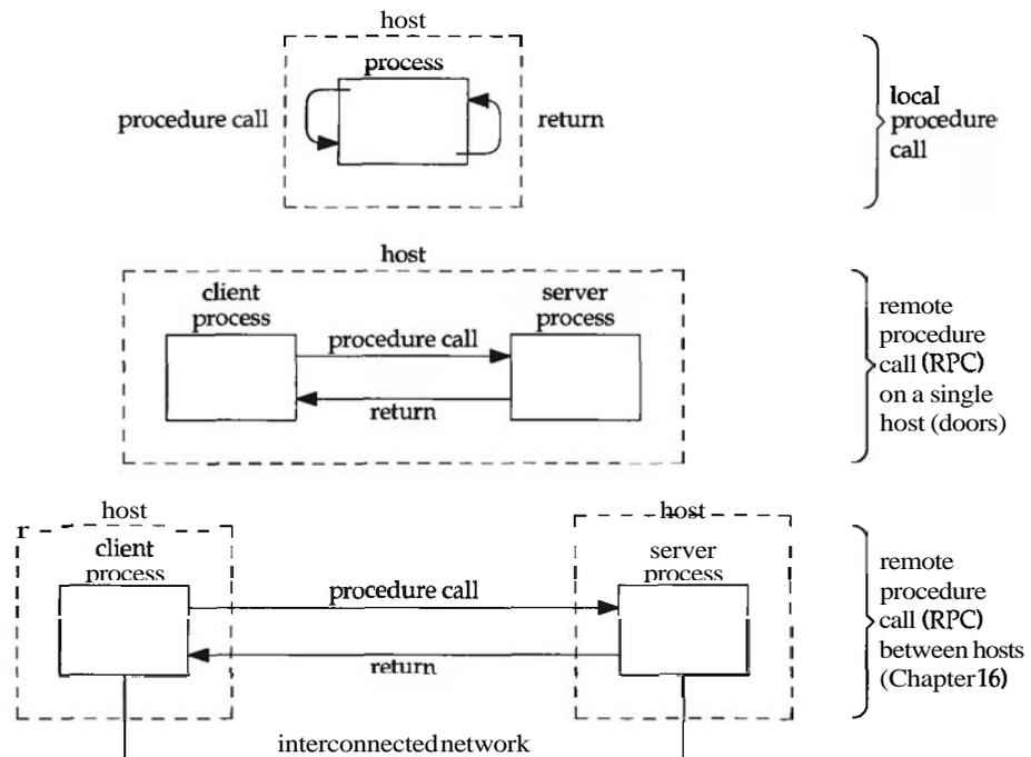
Figure 15.1 Three different types of procedure calls.
