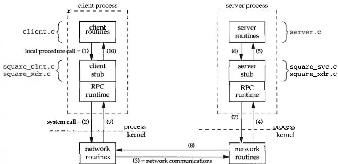
Figure 16.5 Steps involved in a remote procedure call.
