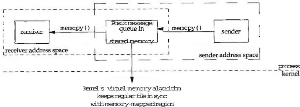
Figure D.8 Sending messages using a Posix message queue implemented using mmap.
