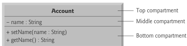
Fig. 7.3 | UML class diagram for class Account of Fig. 7.1.
