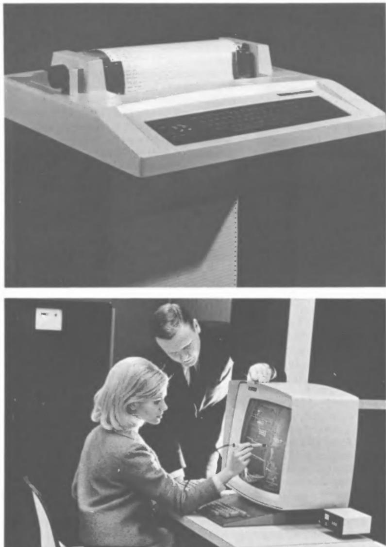
Fig. 1.4 Computer terminals: a standard "hard copy" terminal (top, photo courtesy Digital Equipment Corp.); a graphics terminal (bottom, photo courtesy IBM Corp.).
