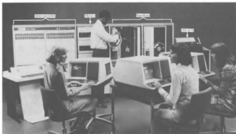
Fig. 1.5 Digital Equipment's VAX-11/780 computer system. (Photo courtesy Digital Equipment Corp.)
