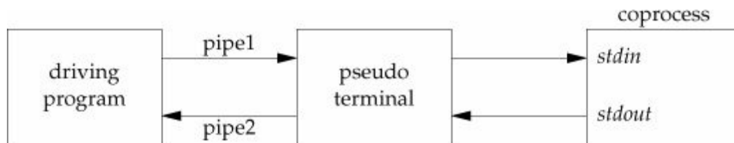
Figure 19.6 Driving a coprocess using a pseudo terminal
