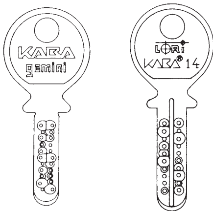
Figure 8.9 Examples of Kaba composite bitted keys. (Lori Corp.)
