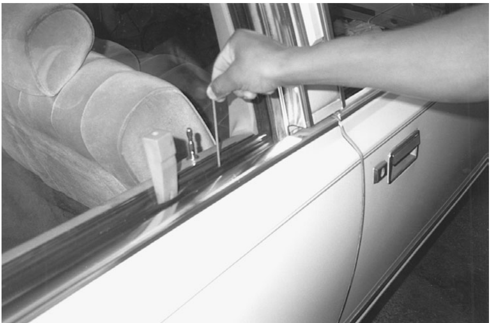
Figure 16.11 When the J tool is below the window, turn it so it is beneath the lock button.
