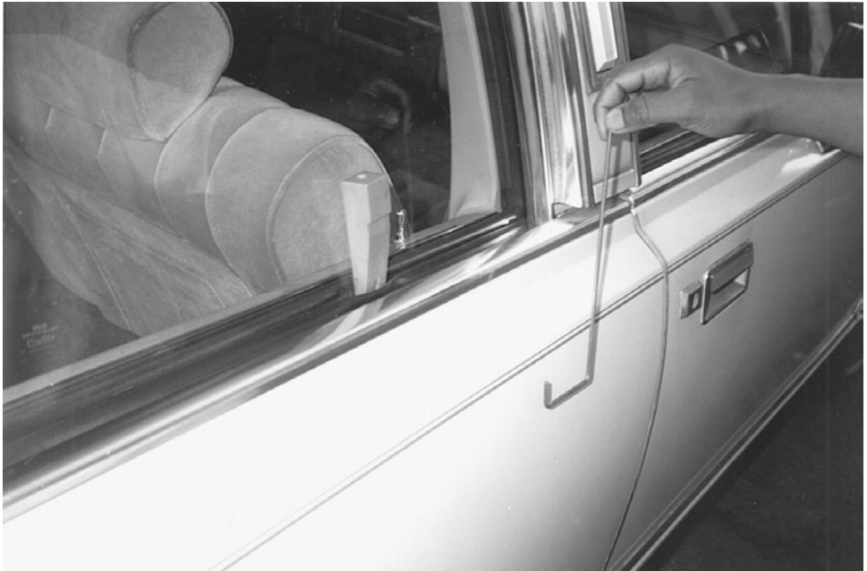
Figure 16.10 The J tool goes within the door near the lock button.
