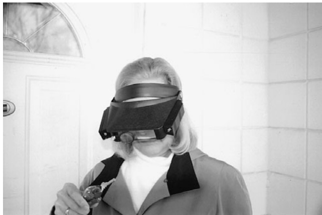
Figure 14.14 Head-mounted magnifying glasses can help you to see impression marks.
