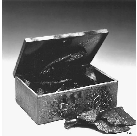
Figure 11.1 A UL-listed fire safe or chest is constructed so that its interior stays below a certain temperature during a fire. Nonrated containers might provide no more fire protection than a metal box offers. (Sentry Group)
