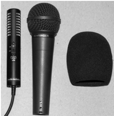
Figure 2-9: Audio-Technica stereo condenser mic, Behringer dynamic mic, and wind sock
