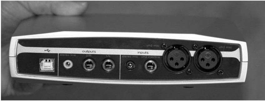
Figure 2-4: M-Audio MobilePre, backside. From left to right: USB jack, stereo line out, 1/4" mono TRS right and left outputs, stereo mic in, Ch. 2 1/4" mono TRS input, Ch. 2 XLR mic jack, Ch. 1 XLR mic jack
