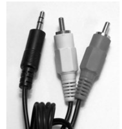
Figure 3-11: Because of the proliferation of 1/8" mini-plugs, this is the workhorse of many a conversion studio.
