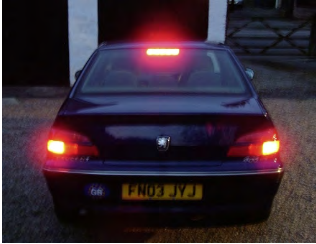
FIG. 1.1 Light emitting diodes have largely taken over the role of brake lights on modern cars and, in many cases, that of parking lights and direction indicators. Headlights, too, are soon likely to take the form of white LEDs. Courtesy of the author.
