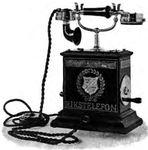
FIG. 8.2 An 1896 Swedish telephone. Compared with the first Bell telephone (Fig 3.1), this shows more than a little evidence of designer influence, though it probably differed very little in its manner of functioning. Courtesy of WikiMedia.
