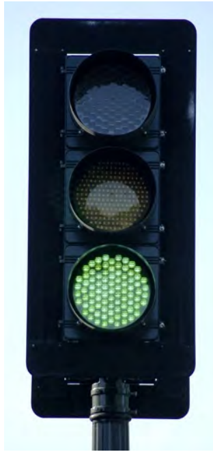
FIG. 7.1 LED traffic lights first appeared in Japan towards the end of the 1990s and are now widely used throughout the developed world. Their improved efficiency and longevity are saving local authorities large amounts of tax-payer's money. Courtesy of iStockphoto, © Harris Shiffman, image 964085.
