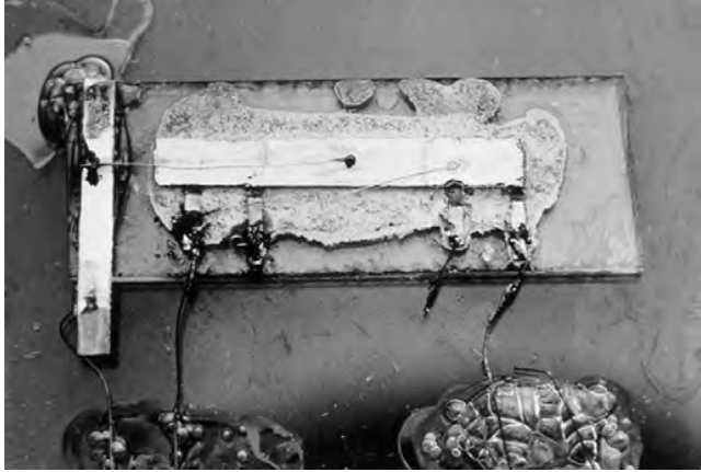
FIG. 4.1 The very first integrated circuit. It was built by Jack Kilby at Texas Instruments in 1958, demonstrating that the functions of resistance, capacitance and gain could all be achieved within a single crystal of germanium. Kilby's circuit lacked an integrated technology for connecting the various components together, making use, instead, of fine copper wires. Courtesy of Texas Instruments Inc.
