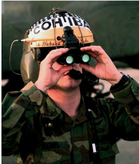
FIG. 9.3 The development of infra-red image tubes which convert invisible radiation into visible took quite a long time. Starting with the discovery of infra-red-sensitive photocathodes in the 1930s, followed by that of the so-called negative-electron-affinity cathode in the 1960s and the invention of the channel plate multiplier at about the same time, it became possible to build small, convenient image tubes which could be fashioned into light-weight night vision goggles as shown in the photograph. Courtesy of WikiMedia.
