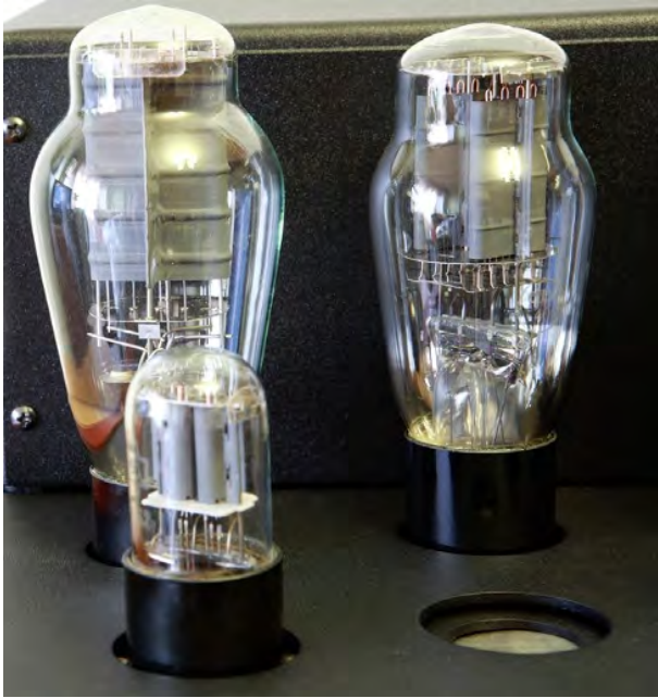
FIG. 2.2 A selection of triode thermionic valves in a valve amplifier. The triode was invented by Lee de Forest in 1906 and was adopted by Bell engineers for use in long-distance telephone communications in the early years of the twentieth century. It enjoyed a long history until competition from the transistor and integrated circuit reduced sales to fairly modest proportions during the 1970s. Courtesy of iStockphoto, © Valeriy Novikov, image 8117713.
