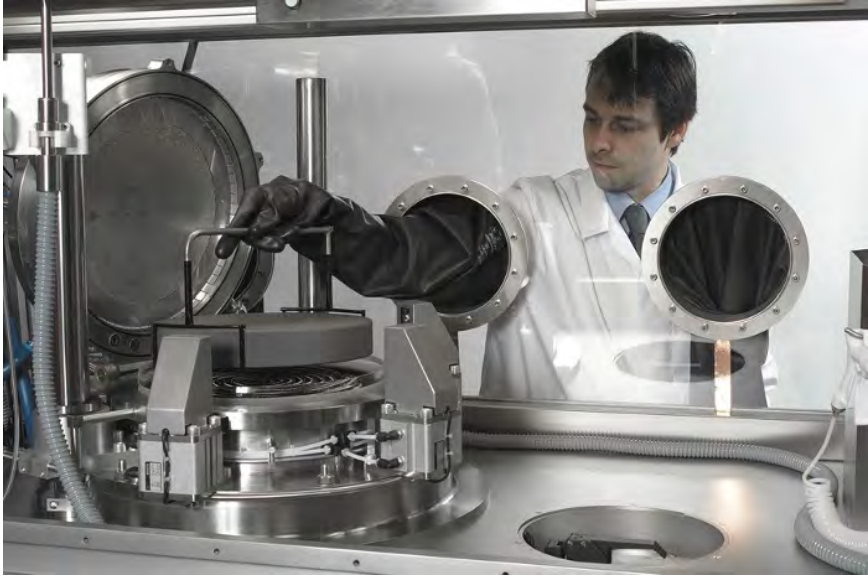
FIG. 6.2 A modern MOVPE (metal-organic vapour-phase epitaxy) machine used to grow thin, single crystal films of III-V semiconductors, such as gallium arsenide and indium phosphide. Courtesy of Aixtron.
