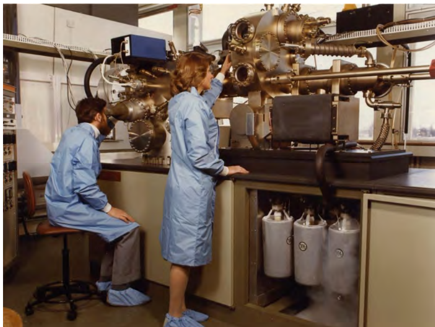
FIG. 6.3 A typical MBE (molecular beam epitaxy) machine used for growing thin layers of single crystal material such as gallium arsenide or aluminium gallium arsenide. It relies on a stainless steel ultra-high vacuum system to keep out unwanted impurity atoms. Courtesy of Tom Foxon.
