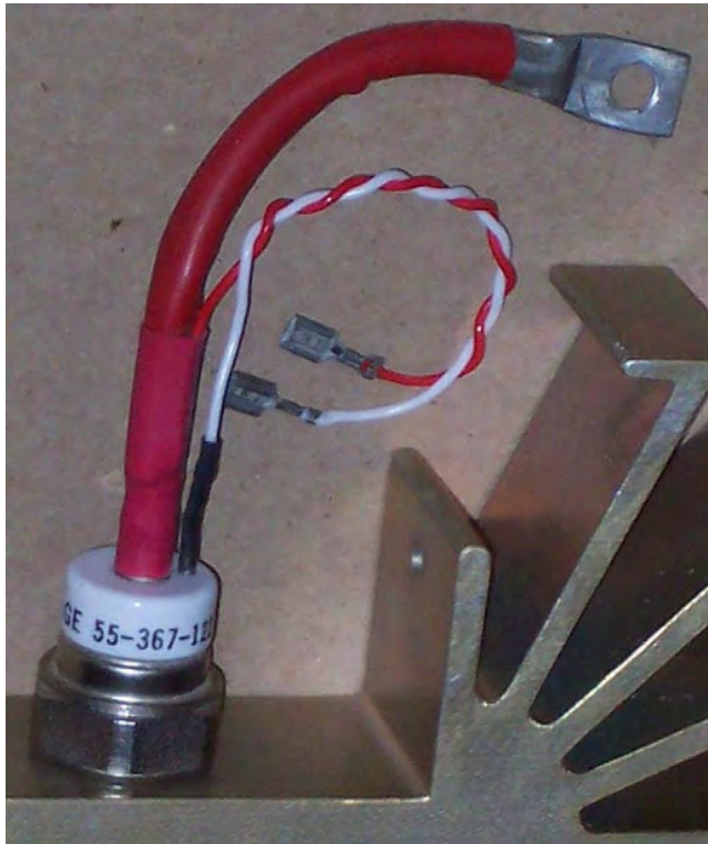
FIG. 4.6 An example of a silicon power device, mounted on heat sink. This is a silicon controlled rectifier (SCR), rated at about 100 amperes, 1200 volts and has a diameter of about half-an-inch. Note the thickness of the current carrying lead, which is appropriate to this large current capacity. Courtesy of WikiMedia.
