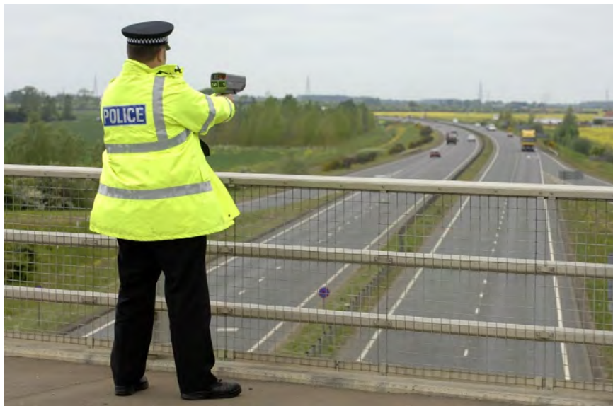
FIG. 5.3 A behind-the-scenes view of a Police radar speed camera in use on one of Britain's motorways. The device makes use of a Gunn diode to generate microwave radiation and measures the Doppler shift in microwave frequency to assess the speed of approaching cars. Courtesy of iStockphoto, image 3366444.
