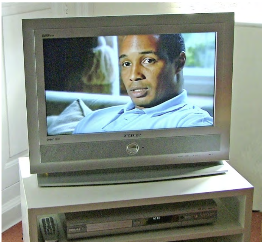
FIG. 10.3 The new millennium saw liquid crystal, flat panel display take over remarkably rapidly from the long-standing cathode ray tube in television and computer display. The picture shows a typical LCDTV set such as has come to dominate most of our living rooms in the twenty-first century. Courtesy of the author.
