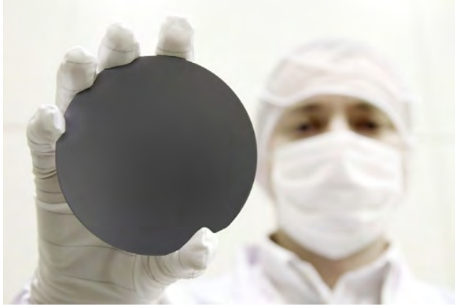
FIG. 1.5 Silicon wafers have grown rapidly in diameter since the introduction of the first integrated circuits in the 1960s. The more chips that can be accommodated on each slice, the less does each one cost. The six-inch wafer shown here is already dwarfed by its more recent counterparts. Courtesy of iStockphoto, © Alexander Gatsenko, image 7822588.
