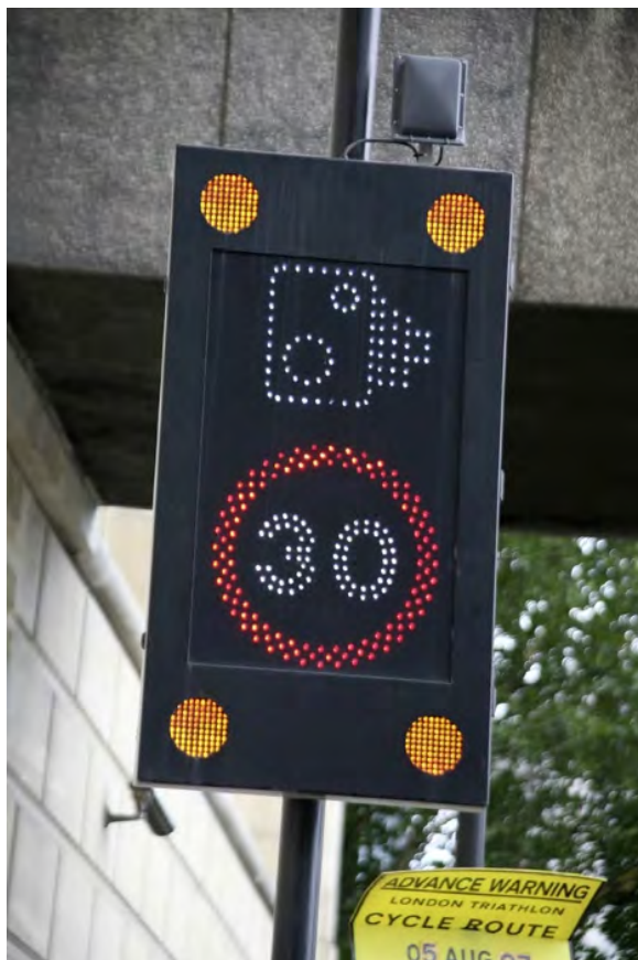
FIG. 7.3 A traffic warning sign using several differently coloured LEDs. Once the idea of using LED traffic lights caught on in the early years of the new millennium, local authorities vied with one another to introduce a wide range of active warning signs, also based on the new high-brightness LEDs. Courtesy of iStockphoto, © Nick Free, image 3967053.
