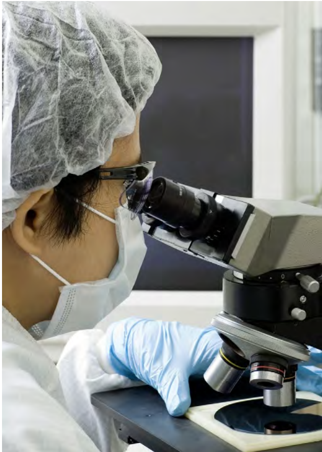
FIG. 4.5 An operator working in a semiconductor clean room. The minimisation of dust particle count is an essential feature of modern integrated circuit manufacture and all personnel are obliged to wear specially washed clothing designed to prevent the shedding of skin or hair. Human beings are far and away the dirtiest components of clean room equipment! Courtesy of iStockphoto. © Eliza Snow, image 2529737.
