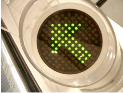
FIG. 7.5 A green LED direction arrow. The inherent brightness of modern LEDs makes them particularly attractive for numerous different types of sign. They catch the eye much better than ordinary painted signs and they can, where necessary, be made to flash on and off to attract attention even more insistently. Courtesy of iStockphoto, © Ulrich Koch, image 117711.
