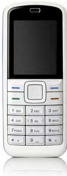
FIG. 6.4 The ubiquitous mobile phone depends for its connections on microwave radiation which is processed by highly sensitive field-effect transistors made from carefully strained thin films of various III-V compound semiconductors. Courtesy of iStockphoto, © Jakub Semeniuk, image 5395519.
