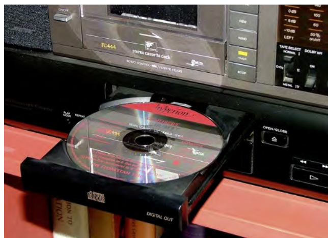
FIG. 5.2 The first major application for the newly developed gallium arsenide laser was as the light source used to read information from a compact disc in the CD player launched by Philips and Sony in 1978. The CD player shown here was manufactured by neither of those companies but is typical of the millions of players produced over subsequent years. Courtesy of the author.
