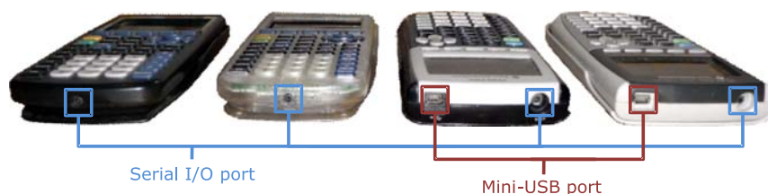
Figure A.9 The serial (I/O) and/or mini-USB ports at the edges of, from left to right, the TI-83+, the TI-83+ Silver Edition, the TI-84+, and the TI-84+ Silver Edition
