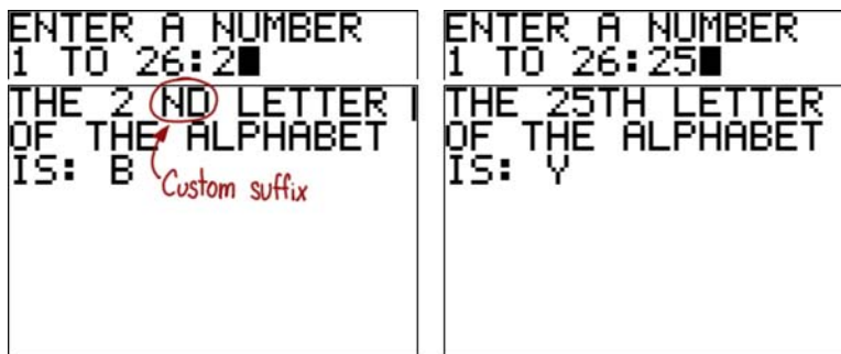
Figure 9.1 Two uses of the sub command to manipulate strings demonstrated in prgmLTRNUM
