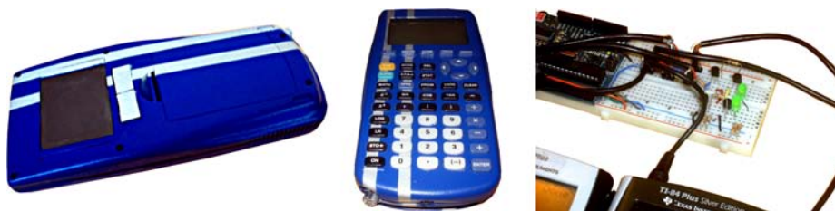
Figure 13.1 Calculator hardware projects in action. The “Ultimate Calculator 2,” left and center, with several hardware modifications; experimenting with calculator networking using CALCnet, at right.
