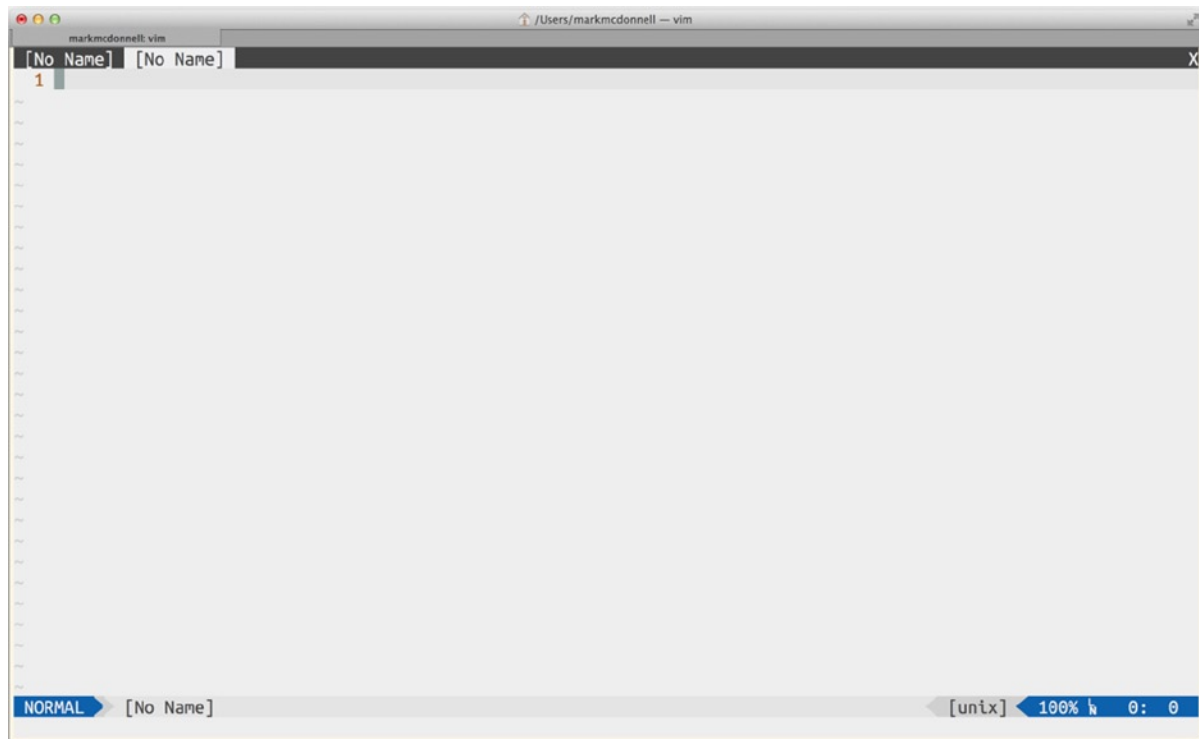
Figure 4-3. Vim's :tabnew command creates a new empty buffer within a new tab
