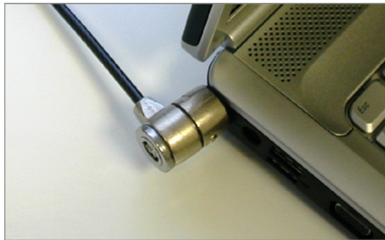
FIGURE 7.16 A cable in the security slot keeps the laptop from being carried away easily.
