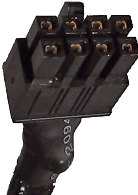
CPU Power Connector (As above)
