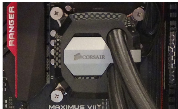
CPU Cooler Block Screwed On Top Of The Processor (Shown above)
