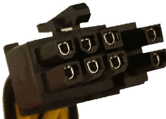
8 (6 + 2) Pin PCI-E Power Connector (Shown above)
