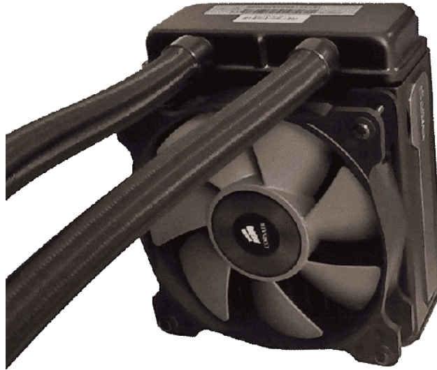
Fan Screwed Onto The Radiator (Shown above)
