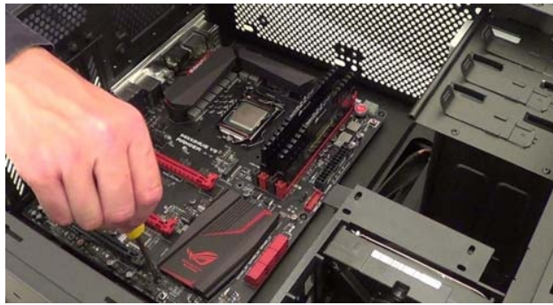
Screwing Down The Motherboard (Shown above)
