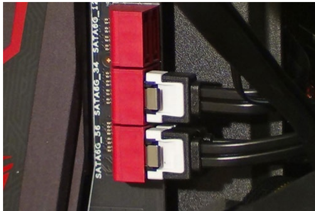
SATA Data Cables Plugged Into The Motherboard (Shown above)
