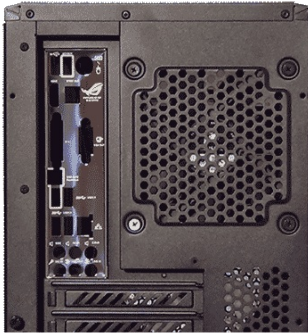
I/O Plate Installed (Back Of Case) (Shown above)
