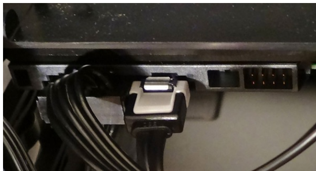
SATA Data Cable Plugged Into The HDD (Shown above)
