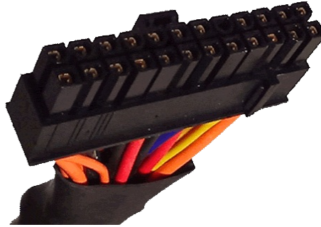
24 pin Motherboard power connector (Shown above)
