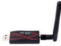
Figure 306. The MetaGeek Wi-Spy DBx adapter listens to RF signals
