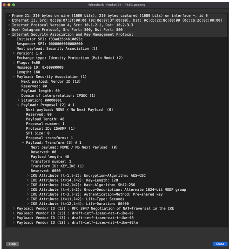
Figure 5-28. Wireshark capture of first Phase 1 packet
