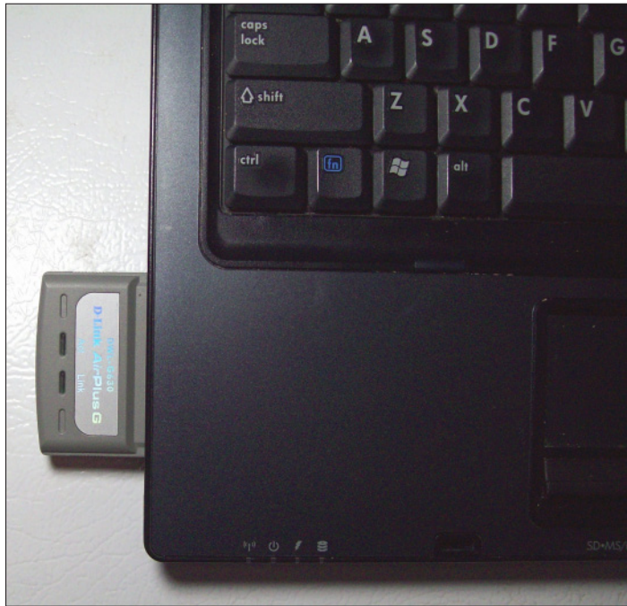
Figure 5-8: A PC Card that's been inserted into a laptop.
