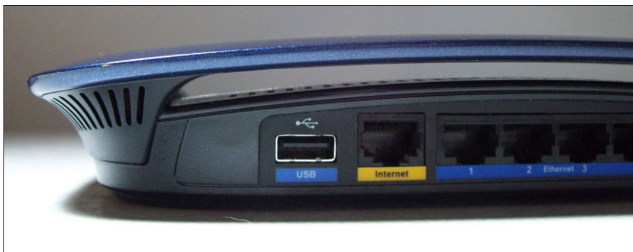
Figure 7-8: A USB port on a router for an external storage device.
