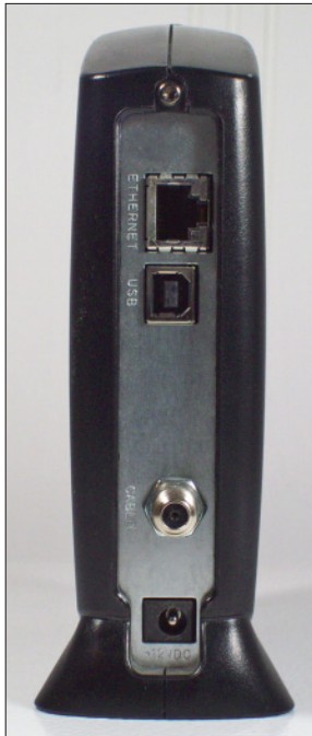
Figure 3-2: Finding the Ethernet jack on a cable modem.
