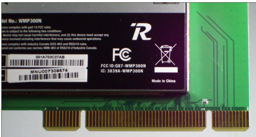
Figure 5-12: The edge connectors on a wireless card.
