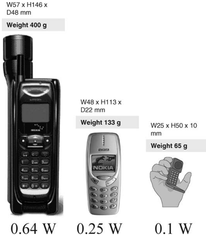
FIGURE 3.2 Power consumption and the size/weight of a mobile terminal.
