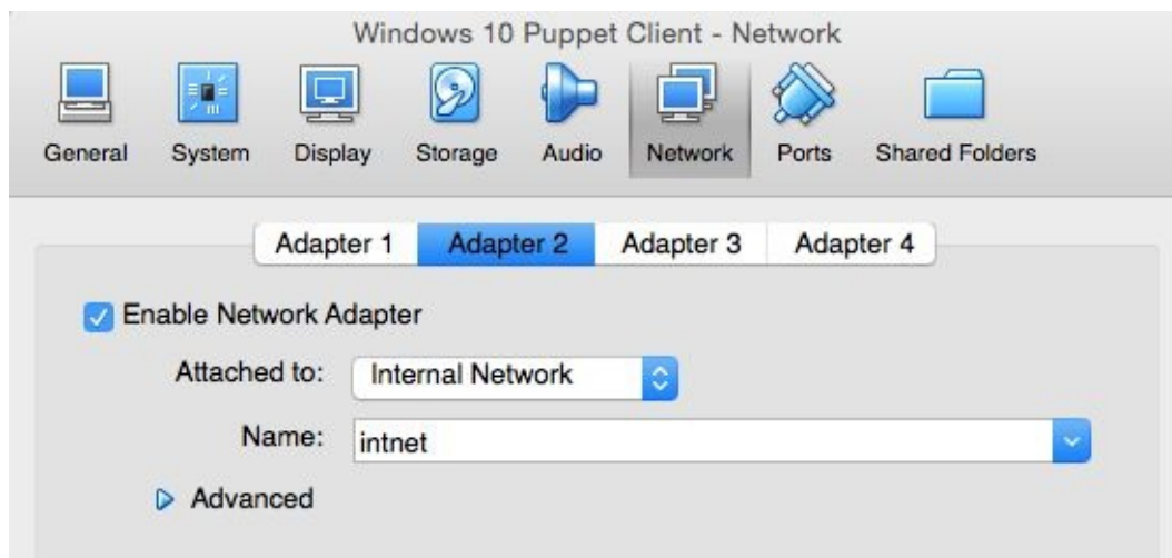
Figure 28-2. Attach Adapter 2 to the Internal Network
