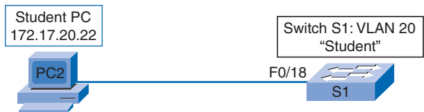
Figure 3-28 Switch Topology for Basic VLAN Configuration
