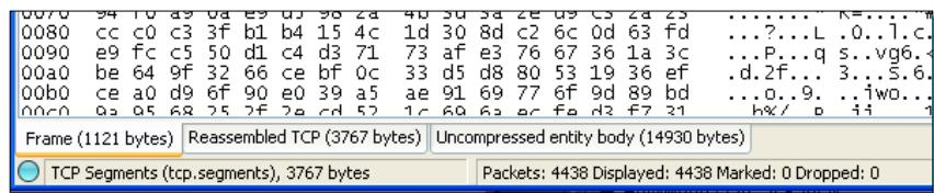
For example, an HTTP GET request (HTML page) can be broken into smaller data packets. Once the transmission is complete, Wireshark reassembles the different packets and creates a single reassembled HTML page. The packet details panel adds extra information (**Reassembled TCP segments**) about the different packet numbers that are reassembled to form the complete set of data.
