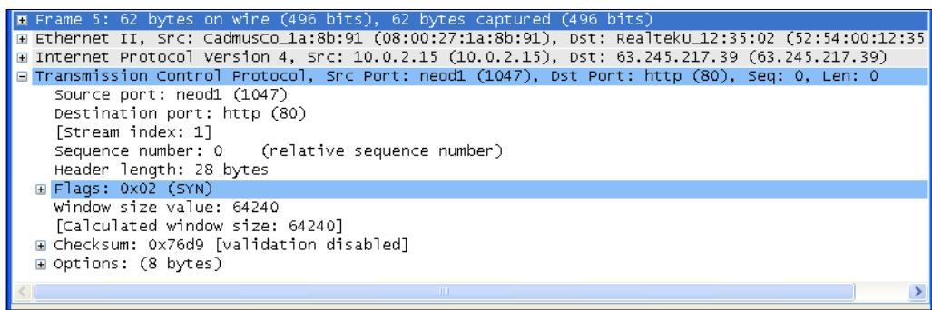
The screenshot shows the Wireshark packet details panel for a selected TCP SYN packet. The panel is organized into a tree structure with expandable and collapsible sections. The expanded sections include:
