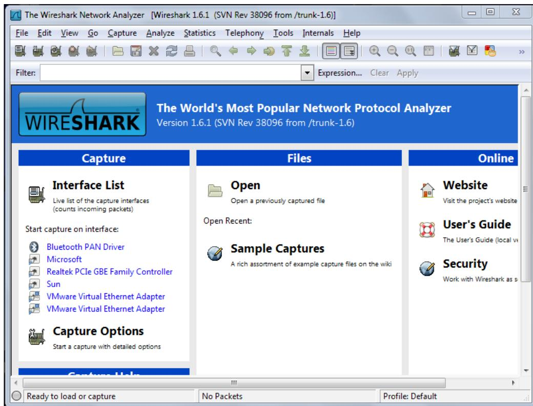
As you can see, the top-left column of the main window displays different capture interfaces under the heading **Interface List**. We can select any interface of our choice to start working with. For example, to capture the LAN traffic flowing across your system, you can choose the default LAN network card installed on your system. Similarly you can select the 802.11 Ethernet adapter for wireless data capture over LAN and so on.
