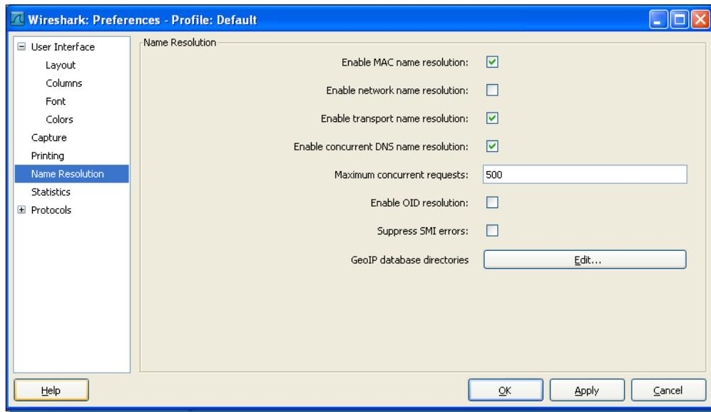
This provides even more advanced options as compared to the previous one. Here we can also provide a GeolP database to Wireshark that can further improve the resolution power of Wireshark by helping it in identifying the packet regions based on its GeolP.
