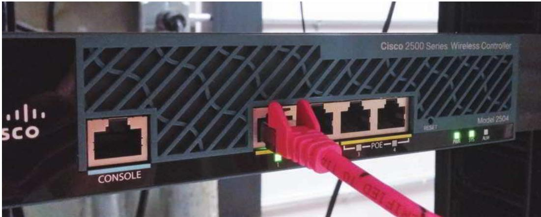
**Figure 6-18** Use a wireless controller to configure, deploy, and manage APs
