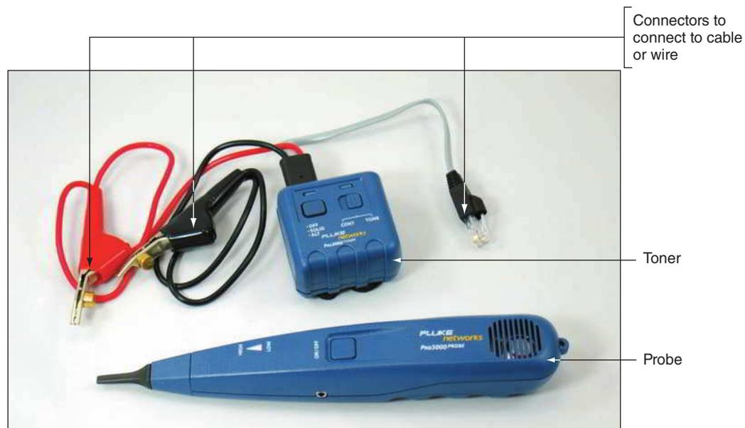
**Figure 5-46** A toner and probe kit by Fluke Corporation
