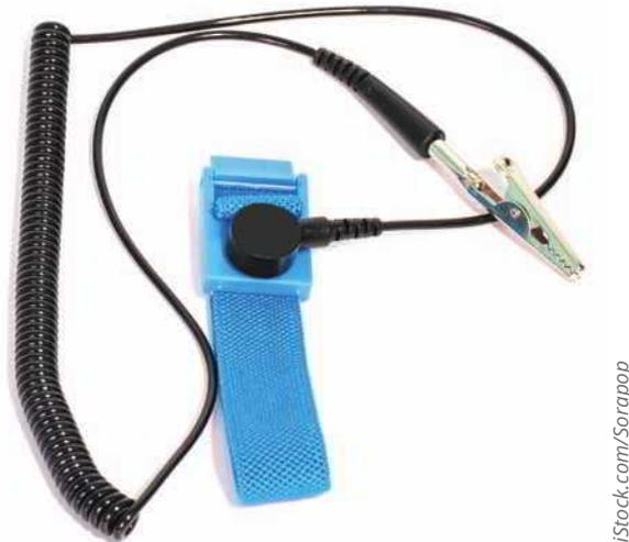
**Figure 1-23** An ESD strap, which protects computer components from ESD, can clip to the side of the computer chassis and eliminate ESD between you and the chassis
