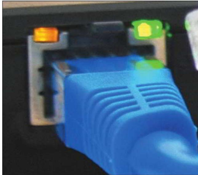
**Figure 5-45** Status indicator lights for an onboard network port
