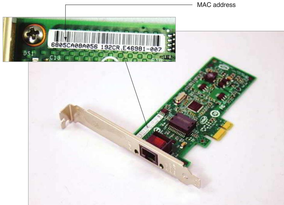
**Figure 1-10** This Intel Gigabit Ethernet adapter, also called a network interface card or NIC, uses a PCIe x1 slot on a motherboard
