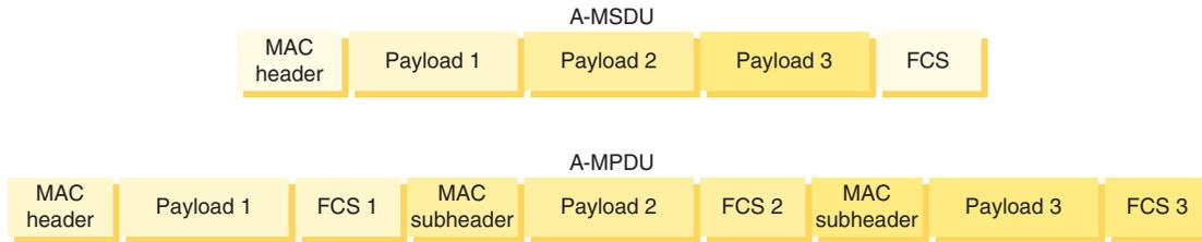
**Figure 6-12** A-MSDU and A-MPDU aggregated frames
