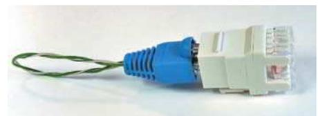
**Figure 5-56** Attach the plug and jack together to protect their connections when storing them
