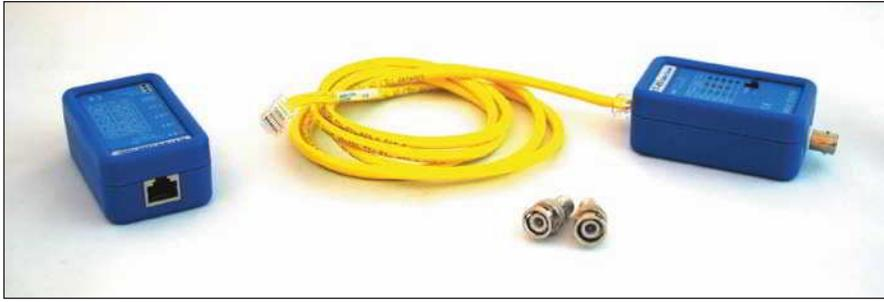
**Figure 5-49** Use a cable tester pair to determine the type of cable and if the cable is good
