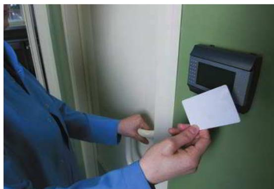
**Figure 10-20** A proximity card does not require physical contact with a proximity reader
