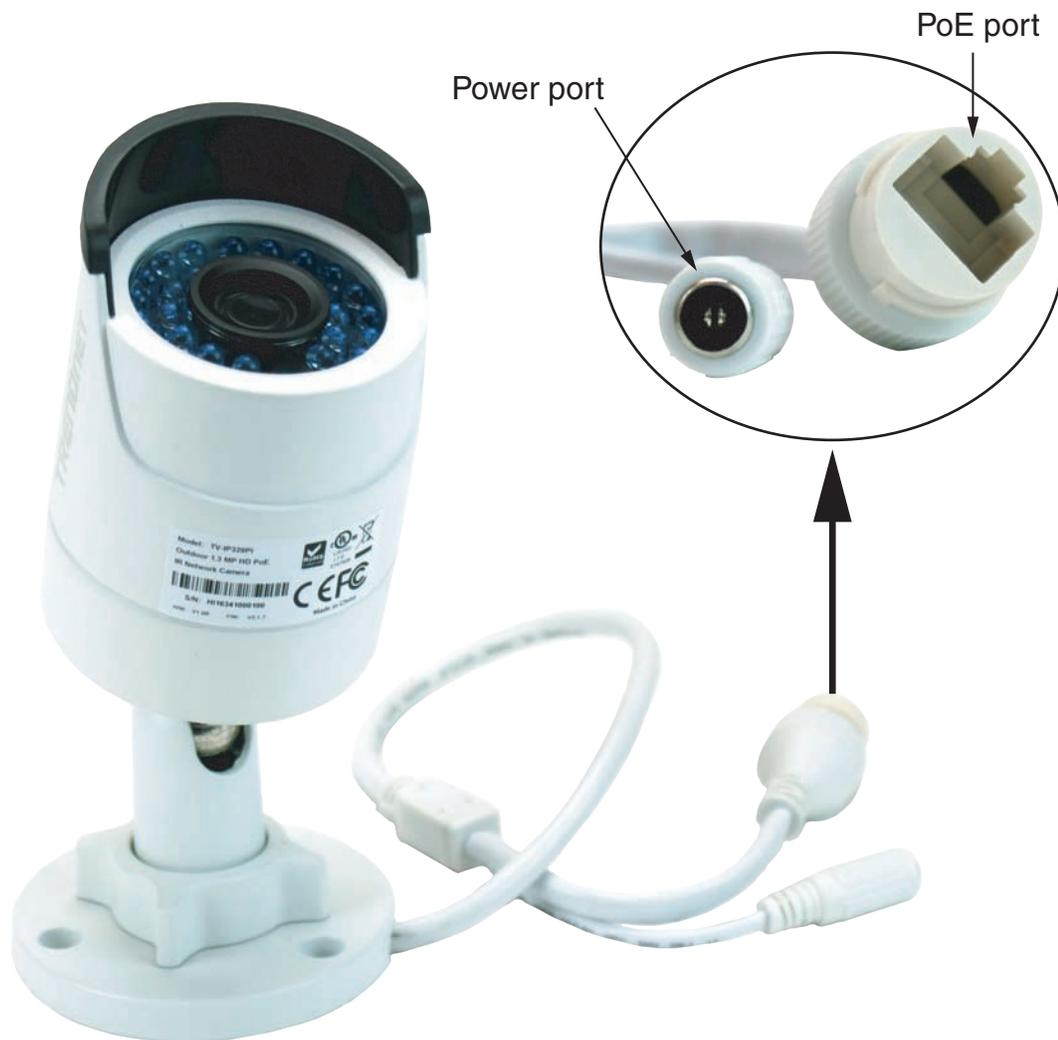
**Figure 5-29** PoE-capable security camera
