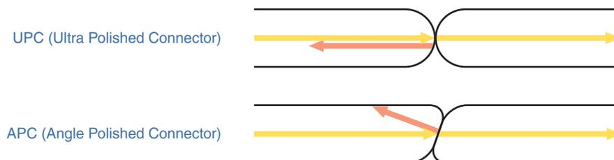
**Figure 5-37** Two types of mechanical connections in fiber-optic connectors
