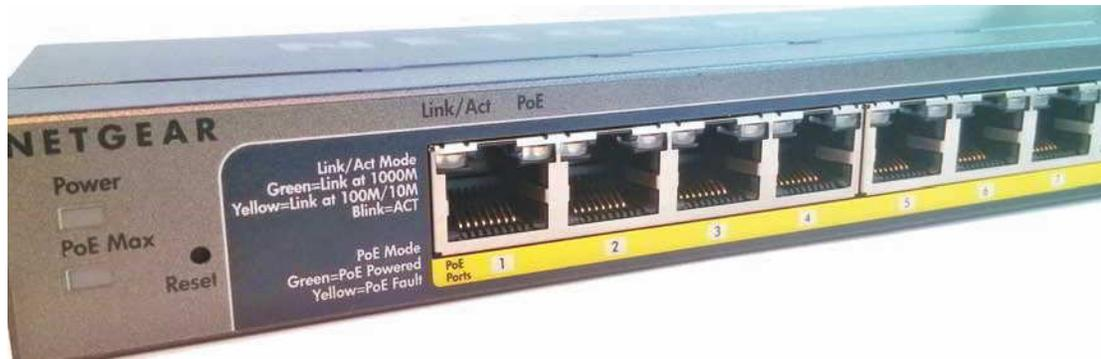
**Figure 5-28** PoE-capable switch
