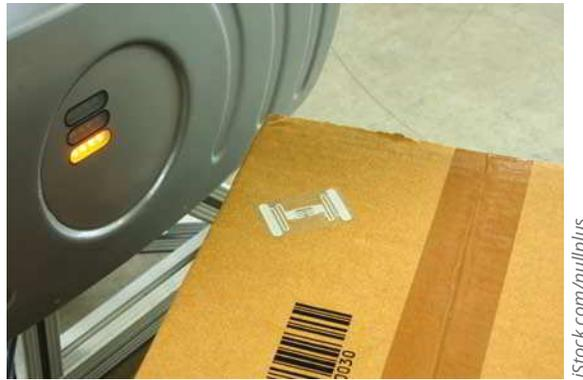
**Figure 10-29** The RFID label on this box allows the delivery service to track its progress
