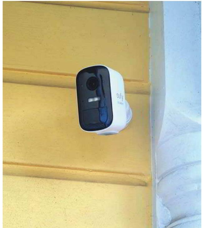
**Figure 6-24** This wireless security camera distinguishes between humans and animals to send more useful alerts and reduce false positives
