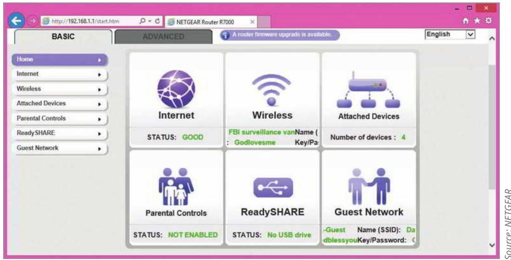
**Figure 6-36** Main page for router firmware setup
