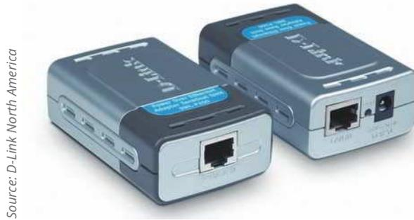
**Figure 5-31** Power and data separately enter this PoE injector through ports shown on the right and exit together through the port shown on the left
