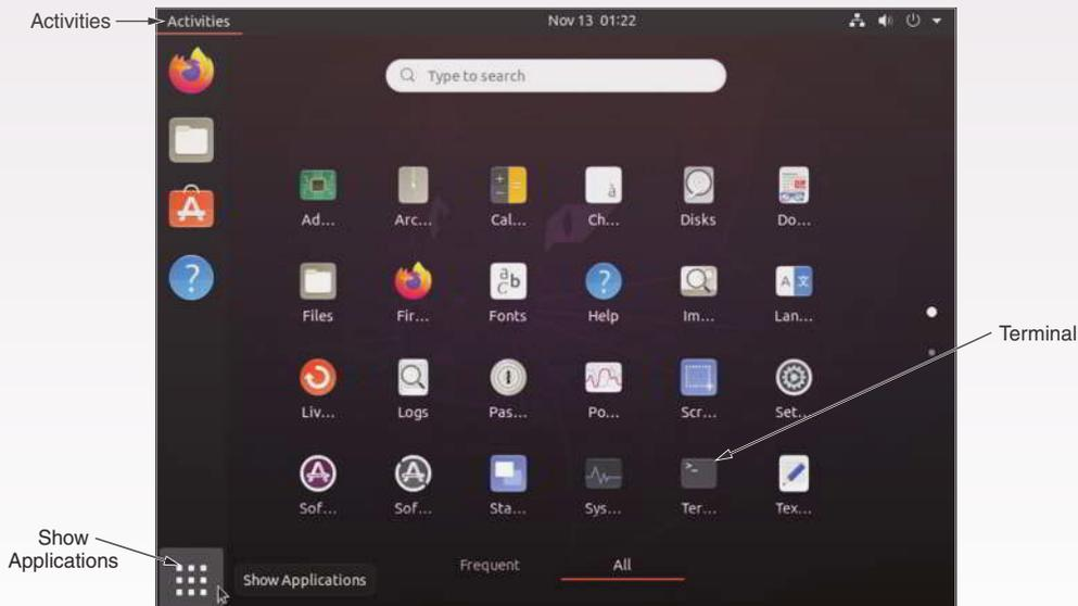
**Figure 3-25** In Ubuntu, Terminal provides a CLI
