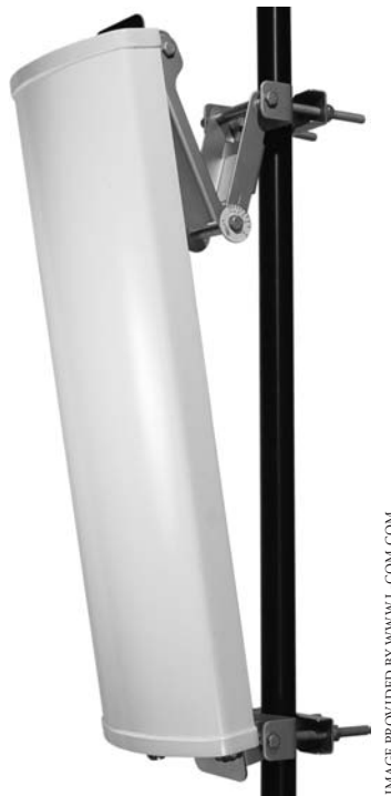
FIGURE 6.12 2.4 GHz 14 dBi 90° sector panel antenna
