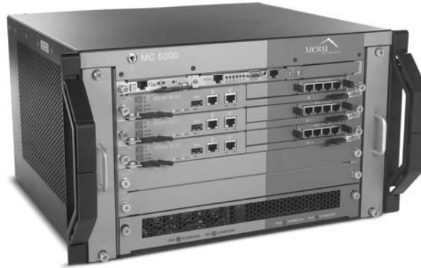
FIGURE 2.14 Meru MC5000 Large Scale Enterprise wireless LAN controller
