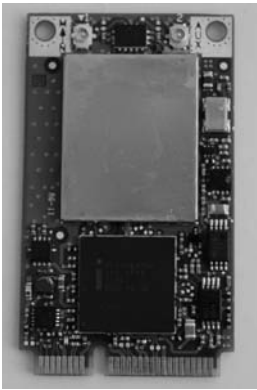
FIGURE 3.10 Intel 3945 IEEE 802.11a/b/g Mini-PCle adapter
