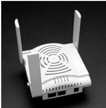
FIGURE 2.8 Aruba Dual-radio 802.11a/n + 802.11b/g/n using 3 antennas
