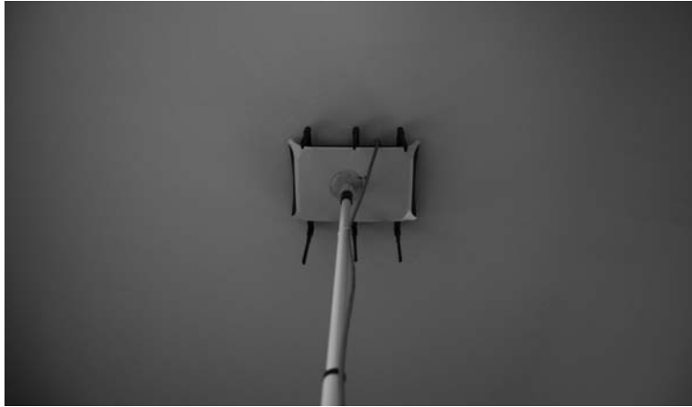
FIGURE 9.8 Access point temporarily mounted using an expandable light pole
