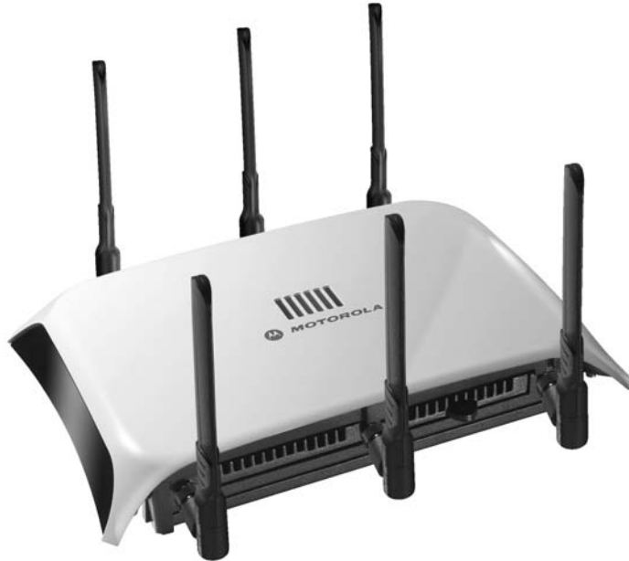
FIGURE 2.6 Motorola AP7131 IEEE 802.11n access point
