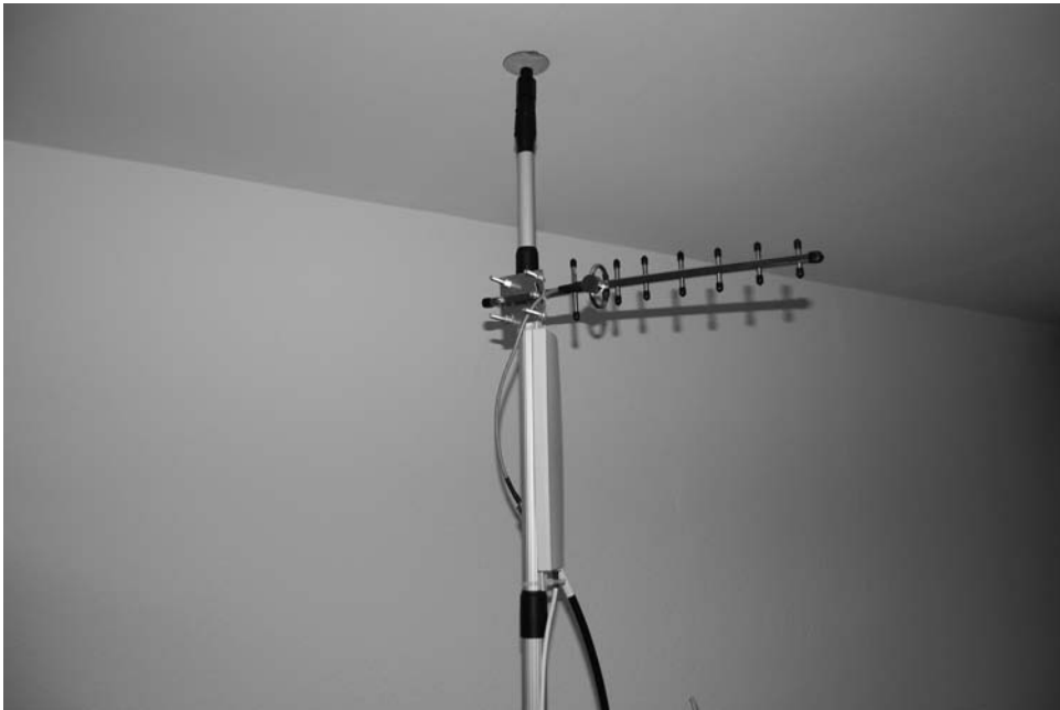
FIGURE 9.17 Expandable light pole used for temporary mounting and testing of a Yagi and Patch antennas
