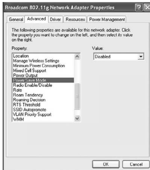
FIGURE 7.26 The driver settings for a Broadcom wireless adapter and power save mode setting
