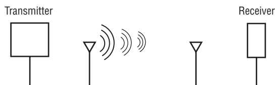
FIGURE 4.3 RF transmitter and receiver. In a wireless LAN the transmitter and receiver could be an access point and client device
