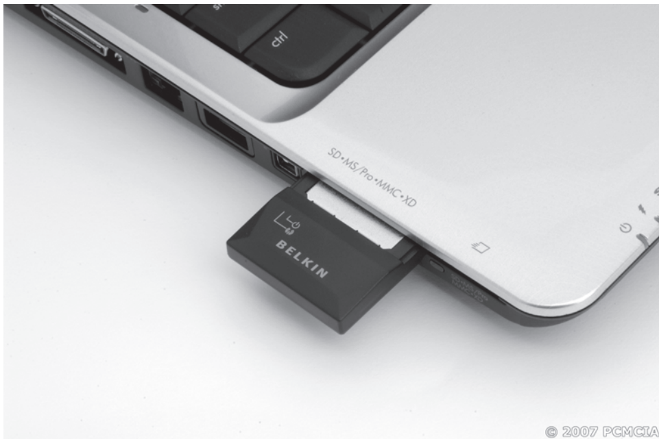
FIGURE 3.4 ExpressCard installed in a notebook computer
